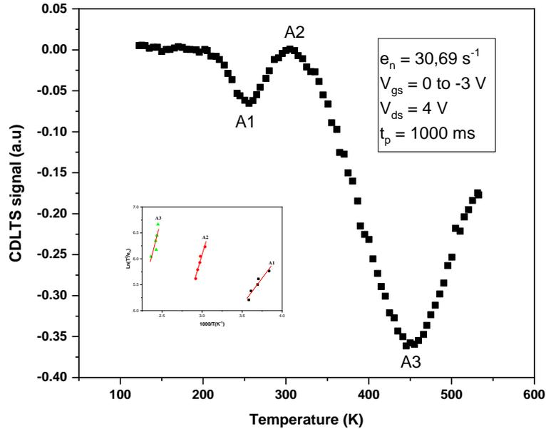
Fig. 3. CDLTS spectra of the AlGaIn/GaN/Si HEMTs. The inset shows the signatures of the traps.
