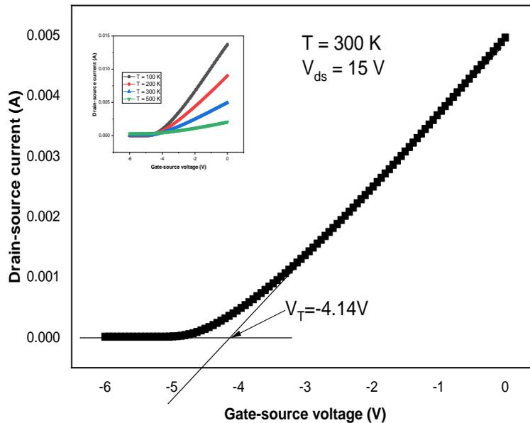
Fig. 2. Transfer characteristics of the AlGaIn/GaN/Si HEMT devices.
