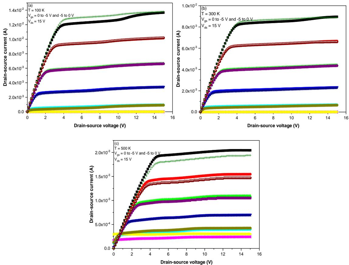
Fig. 1. Direct-current characteristics of the AlGaN/GaN/Si HEMTs at different  $V_{\text{gs}}$  and various temperature.
