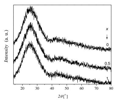
Fig. 1- X- Ray diffactograms of the system  $(1-x)(50P_2O_548CaO_2ZrO_2)$  with x = 0; 1 and 3 mol %Ag.
