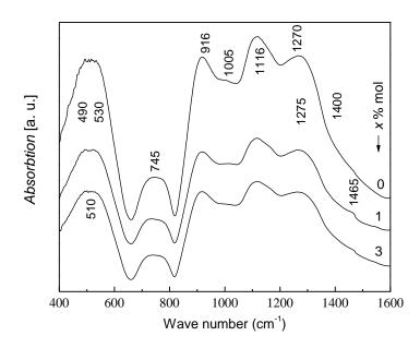
Fig. 2- FT-IR spectra characteristic of vitreous  $(1-x)(50P_2O_548CaO_2ZrO_2)$  with x = 0; 1 and 3 mol %Ag.
