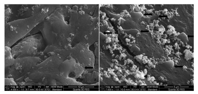
Fig. 6-SEM images at 10µm scale bar (fig.6a) and 5µm scale bar (fig.6b), show glass particles surrounded by the fibroblasts.
