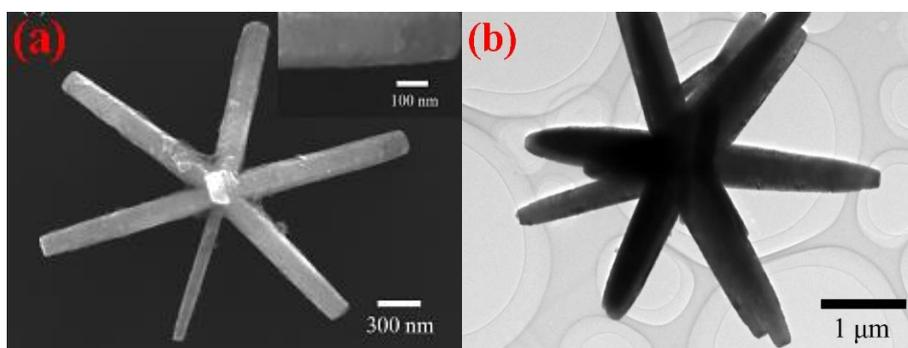
Fig. 5. (a-b): SEM and TEM images of flower-like NC of Pt-ZO [Reprinted (adapted) with permission from (Ref. 106). Copyright (2010) American Chemical Society].
