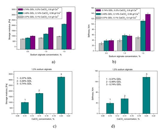
Fig.3 Dependence of storage modulus (a), stiffness (b) and loss modulus (c) of alginate hydrogels by the reactants concentrations
