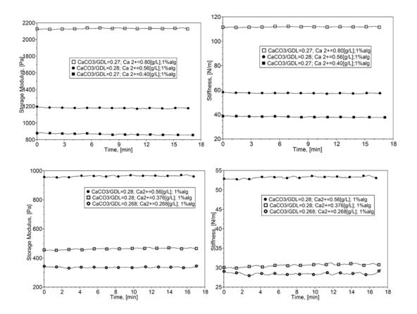
Fig.4. Dependence of the handling consistency by the reactants ratios. Storage modulus (left) and stiffness (right), at 1 Hz for 20 min.
