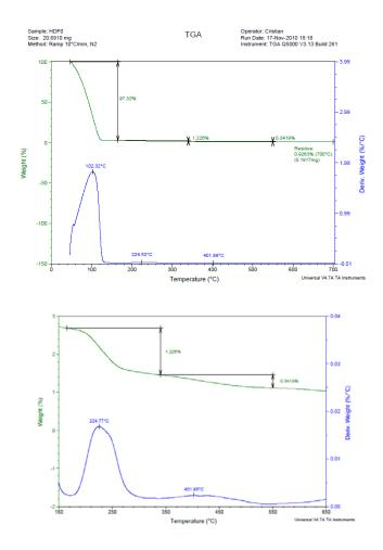
Fig.7. DTA/TGA curves of the studied hydrogels
