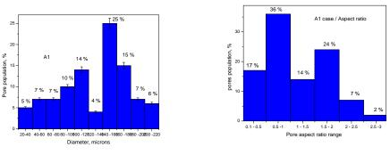
c) d) Fig.8 The morphology of the bead type hydrogels obtained by dropping a CaCl<sub>2</sub> solution in a sodium alginate one (a) and those of the hydrogels obtained with CaCO<sub>3</sub> – GDL system (b, c, d). The pores population distribution considering the diameter range (c) and aspect ratio range (d)
