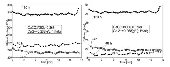
*Fig.2 Time variation of storage modulus and stiffness of hydrogels that has not been washed after crosslinking (stability dynamo- mechanical test at 1 Hz and 37* <sup>0</sup>*C)*
