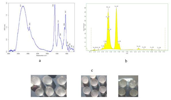
*Fig.1 FTIR spectrum (a) and EDXRF spectrum (b) of layered shaped calcium alginate hydrogel (photo - c) obtained in distilled water, in physiological conditions (3 h, at 37°C in oven)*
