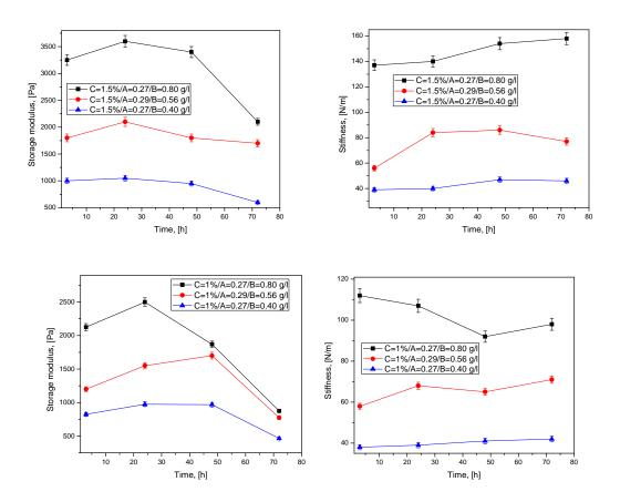
Fig.5. Time dependence of storage modulus and stiffness of the studied hydrogels by the reactants concentrations (A = [CaCO3]/[GDL]; B = [Ca2+](g/l); C = [alginate solution concentrations])
