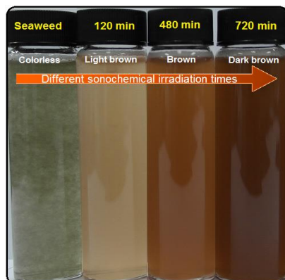
Fig. 1. Photograph of K. alvarezii and Ag-NPs/ K. alvarezii suspension at different sonochemical irradiation times.
