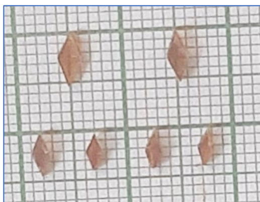
Fig. 1. The grown crystal of the compound 4-nitroaniline picric acid.
