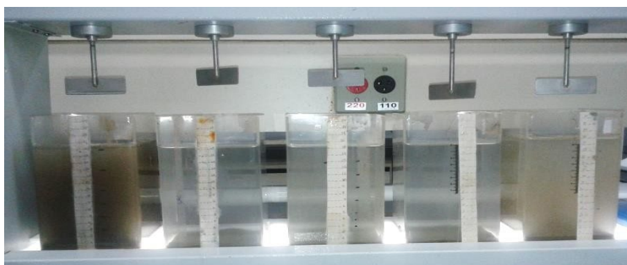
Fig. 7. Ni tailings flocculation jar test.
