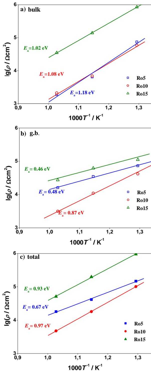
Fig. 4. Arrhenius plots for the total electrolyte resistivity (a), bulk (b) and grain boundaries (c) resistivity for samples S1 (■), S2 (●) and S3 (▲)
