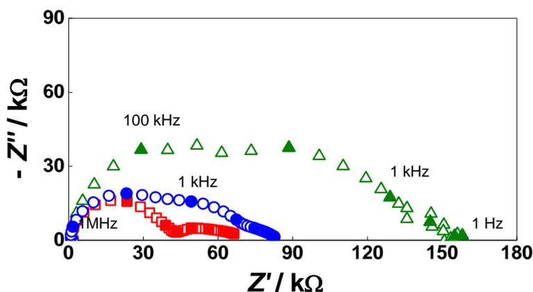
Fig. 3. Complex plane impedance diagrams of samples S1 (●), S2 (■) and S3 (▲) at temperature 500 °C
