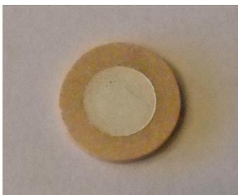
Fig. 1. Sample with silver electrodes used for electrochemical investigation
