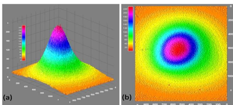
*Fig. 5. Random lasing (one-shot) far field emission intensity profile from a micro-capillary in above threshold energy conditions. (a) 3D emission intensity profile. (b) 2D emission intensity profile*
