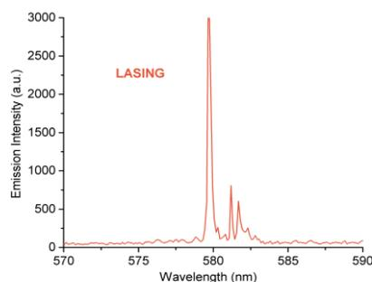
*Fig. 3. Random lasing spectrum from the capillary sample (each lasing mode has a FWHM of ca. 0.5 nm)*
