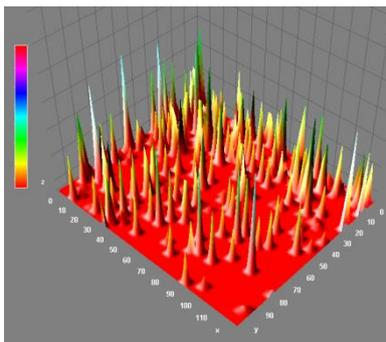
*Fig. 6. High resolution random lasing (one-shot) 3D far field emission intensity profile (acquired from a wedge sample cell excited in the micro array configuration, in above threshold energy conditions).*
