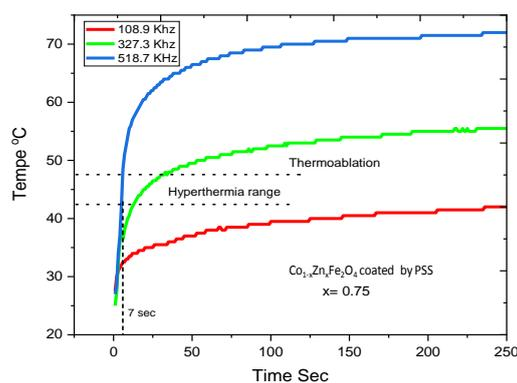
Fig. 7. RF Heating curve of  $\text{Co}_{1-x}\text{Zn}_x\text{Fe}_2\text{O}_4$  by 3 frequencies ( $x=0.75$ ).
