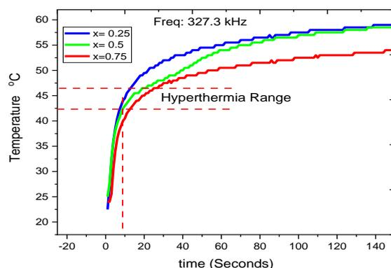
Fig. 8. RF Heating curve of  $Co_{1-x}Zn_xFe_2O_4$  at 327.7 kHz ( $x = 0.25, 0.5, .75$ ).
