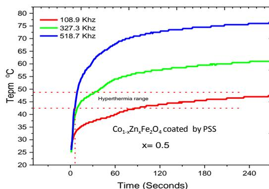
Fig. 6. RF Heating curve of  $\text{Co}_{1-x}\text{Zn}_x\text{Fe}_2\text{O}_4$  by 3 frequencies ( $x=0.5$ ).
