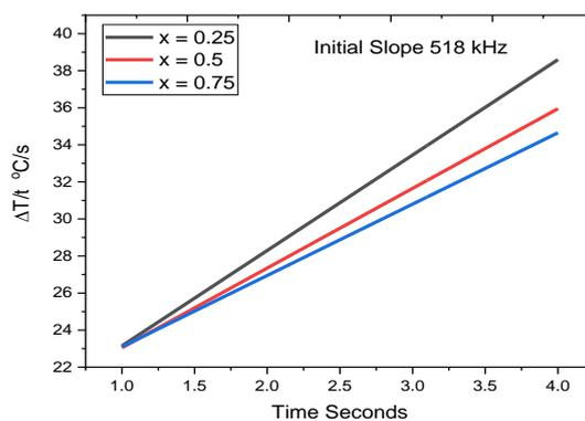
Fig. 11. Initial slopes of  $\Delta T/t$  of three sample for Freq 518.7 kHz.
