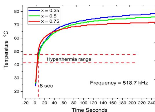
Fig. 9. RF Heating curve of  $Co_{1-x}Zn_xFe_2O_4$  at 518.7 kHz ( $x = 0.25, 0.5, 0.75$ ).
