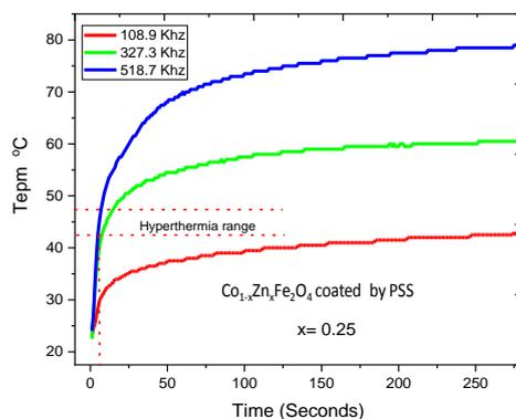
Fig. 5. RF Heating curve of  $\text{Co}_{1-x}\text{Zn}_x\text{Fe}_2\text{O}_4$  by 3 frequencies ( $x=0.25$ ).
