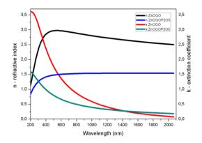
Fig. 9. The refractive index and extinction coefficient of ZnOGO and ZnOP<sub>2</sub>O<sub>5</sub>GO thin film on Glass substrate. The thickness of the film was 433nm ± 17 nm. The measured results were obtained from an ellipsometer within the range of 190-2100 nm (UVISEL, Horiba Jobin Yvon, France).
