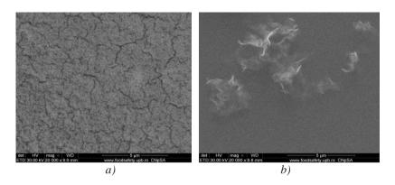
Fig. 1. (a) SEM surface view of ZnOGO and (b) ZnOP<sub>2</sub>O<sub>5</sub>GO thin films deposited on Glass substrate with magnification of 20000x.
