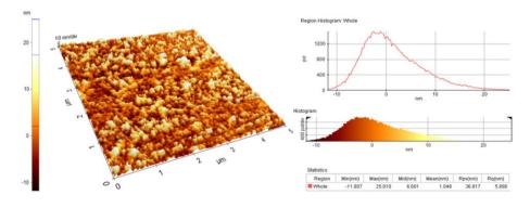
Fig. 3. AFM image of ZnO/GO thin film surface deposited on Glass substrate.
