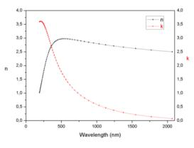
Fig.5. The refractive index and extinction coefficient of ZnO/GO thin film. The thickness of the film was 444nm ± 13 nm. The measured results were obtained from an ellipsometer within the range of 190-2100 nm (UVISEL, Horiba Jobin Yvon, France).
