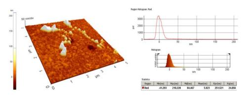
Fig. 6. AFM image of ZnO/P<sub>2</sub>O<sub>5</sub>/GO thin film surface deposited on glass substrate.
