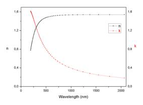
Fig. 8. The refractive index and extinction coefficient of  $ZnOP_2O_5GO$  thin film. The thickness of the film was 433nm ± 17 nm. The measured results were obtained from an ellipsometer within the range of 190-2100 nm (UVISEL, Horiba Jobin Yvon, France).
