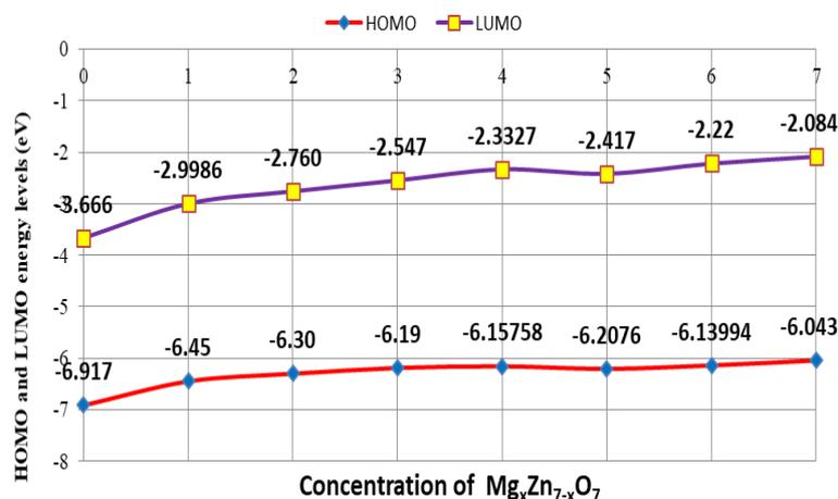
Fig. 3. The HOMO and LUMO of  $Mg_xZn_{7-x}O_7$  as a function of Mg concentration.
