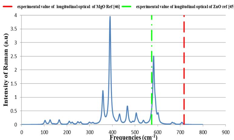
Fig. 5. (b) The Raman spectra of  $Mg_3Zn_4O_7$  compared to the experimental value of LO of MgO and ZnO wurzite.
