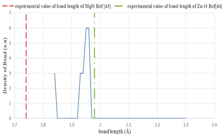
Fig. 4. The density, of bond of  $Mg_3Zn_4O_7$  compare with experimental, value of bond lengths of Zn-O and Mg- O.
