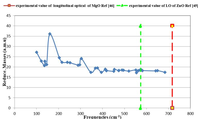
Fig. 6. (b) The reduced masses of  $Mg_3Zn_4O_7$  compared to the experimental value of LO of MgO and ZnO wurzite.
