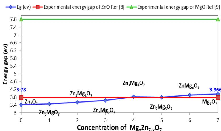
Fig. 2. The band gap of  $Mg_xZn_{7-x}O_7$  as a function of Mg concentration and compared with the experimental values.
