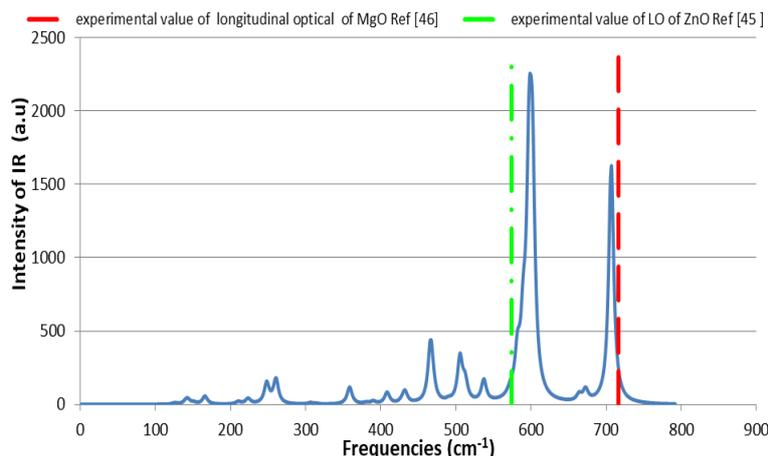
Fig. 5. (a) The IR spectra of  $Mg_3Zn_4O_7$  compared to the experimental value of LO of MgO and ZnO wurzite.
