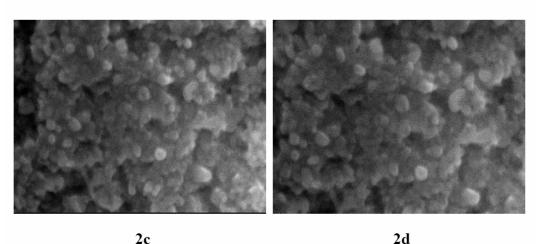
Fig. 2. TEM micrograph 2a(25K); 2b (50K); 2c(60K); 2d(75K) of silver nanoparticles synthesized by the reaction of 1mM silver nitrate with A.paniculata antibiofilm extract.
