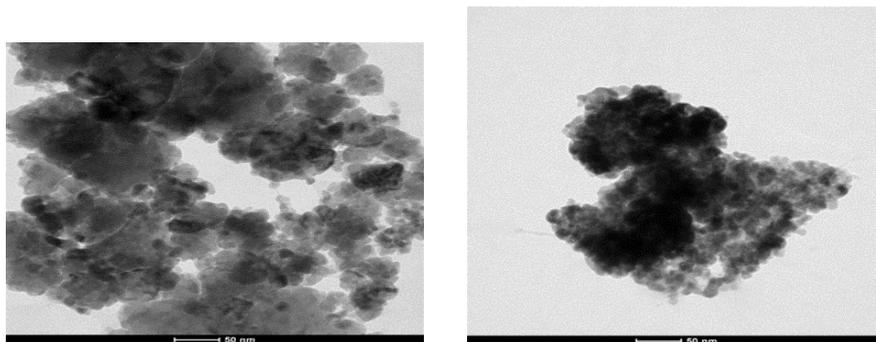
Fig. 3. TEM images of lead selenide quantum dots encapsulated with chitosan
