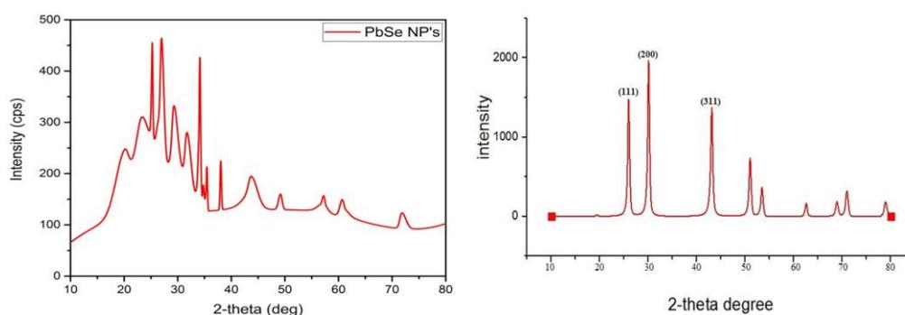
Fig. 5. X-ray diffraction results of lead selenide quantum dots a) PbSe quantum dots
