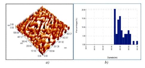
Fig. 4. (a) AFM images of PS prepared by ECE technique with a constant time 20 min. (b) Schematic Granularity Accumulation Distribution.
