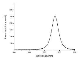
Fig. 5. PL spectrum of ps prepared by ECE technique with a constant time 20min
