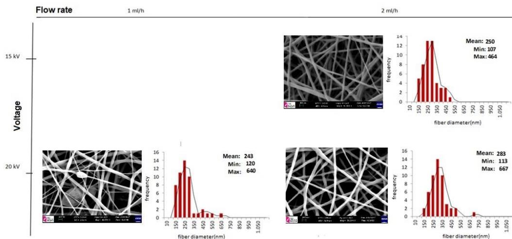
Fig. 2. Morphology and average fiber diameter of PCL/SF nanofibers produced at voltages of 15 and 20 kVs and flow rates of 1 and 2 ml/h (50000 X).
