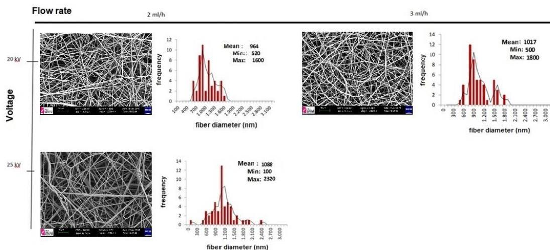
Fig. 3. Morphology and average fiber diameter of curcumin loaded PCL/SF nanofibers produced at voltages of 20 and 25 kVs and flow rates of 2 and 3 ml/h (50000 X).
