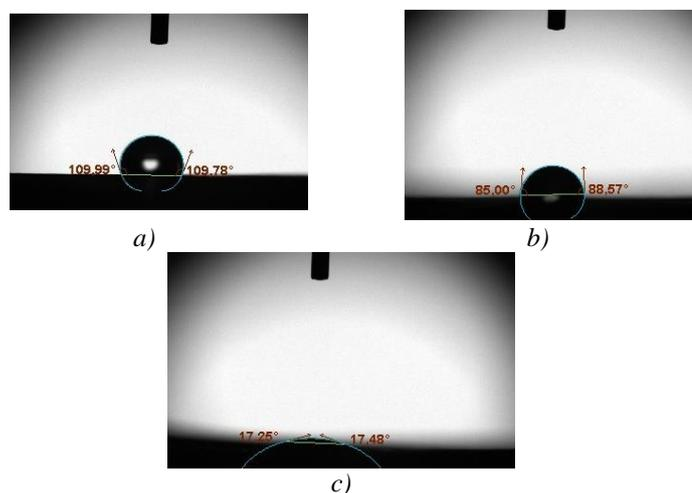
Fig. 5. Water contact angle a) PCL, b) PCL/ SF c) Curcumin loaded PCL/SF.
