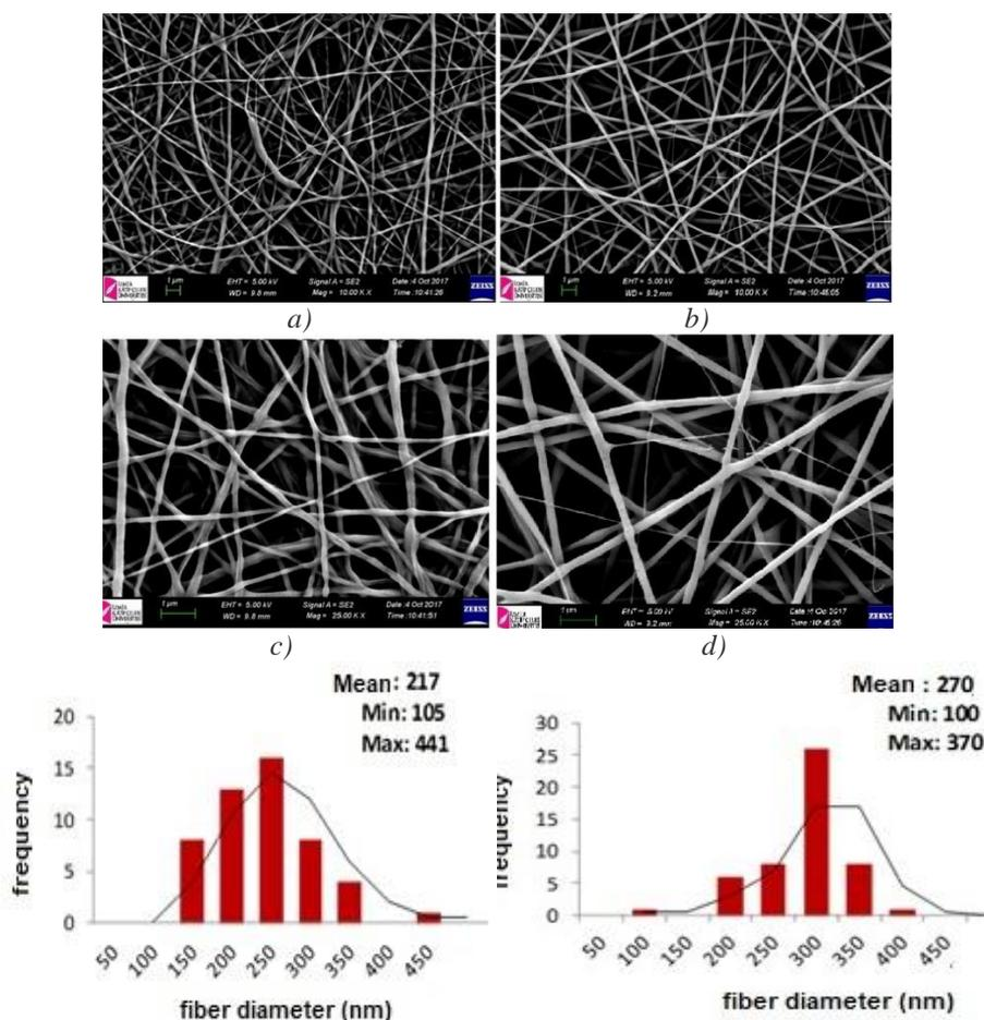
Fig. 1. Morphology and average fiber diameter of PCL nanofibers. 10% PCL nanofibers flow rate: 2 ml/h Voltage: 15 kV (a) 10000 X (b) 25000 X; 15% PCL nanofibers flow rate: 2 ml/h Voltage: 20 kV (c) 10000 X (d) 25000 X
