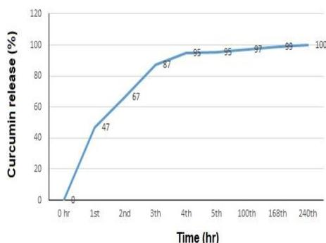
Fig. 6. Release profile of curcumin loaded PCL/SF nanofibers.
