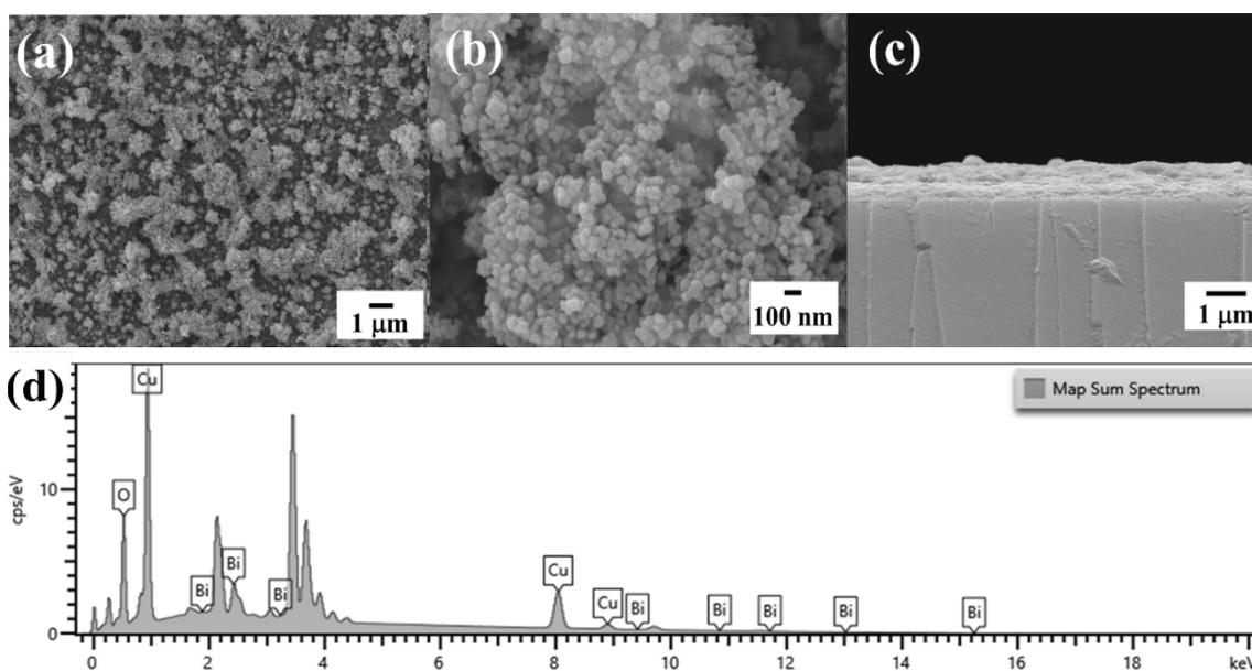
Fig. 2. SEM image of  $\text{CuBi}_2\text{O}_4$  synthesized by the electrochemical deposition.
