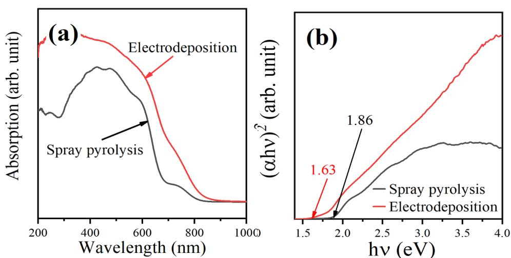
Fig. 4. (a) UV visible absorption spectra and (b) Tauc plot of  $\text{CuBi}_2\text{O}_4$  fabricated by different methods.
