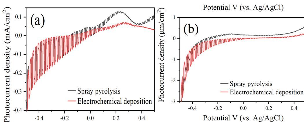
Fig. 5. CLV of  $\text{CuBi}_2\text{O}_4$  fabricated by electrochemical deposition method and spray pyrolysis method were tested in (a)  $0.5 \text{ M Na}_2\text{SO}_3$  and (b)  $0.5 \text{ M NaHCO}_3$  electrolytes.
