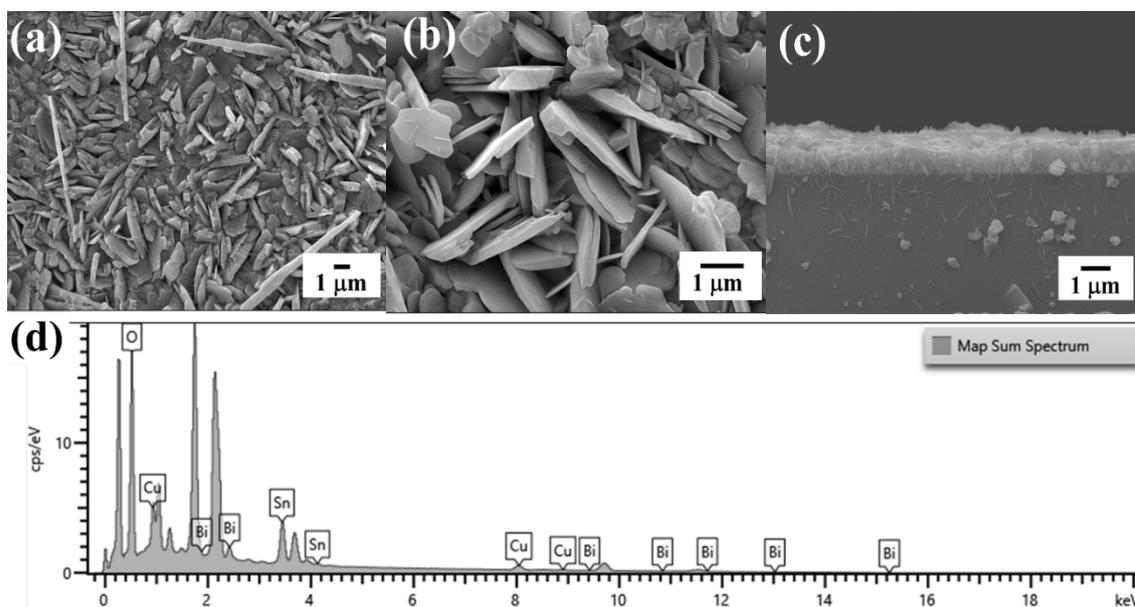
Fig. 3. SEM image of  $\text{CuBi}_2\text{O}_4$  synthesized by the spray pyrolysis deposition.
