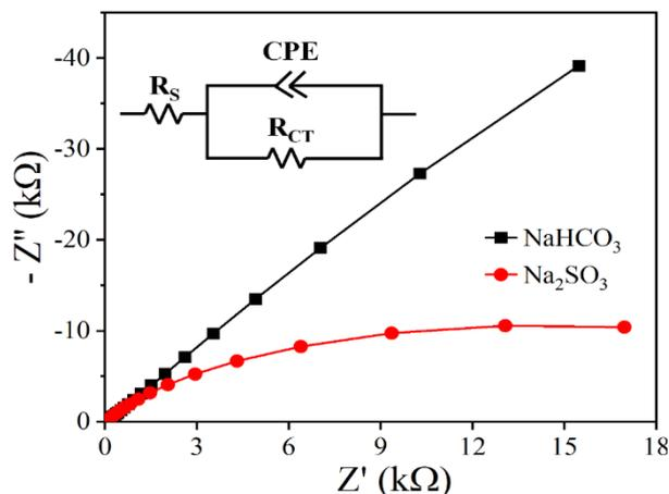
Fig. 6. Nyquist plot of  $\text{CuBi}_2\text{O}_4$  photocathode tested at applied  $-0.3\text{ V}$  (vs.  $\text{Ag}/\text{AgCl}$ ) under visible light illumination.
