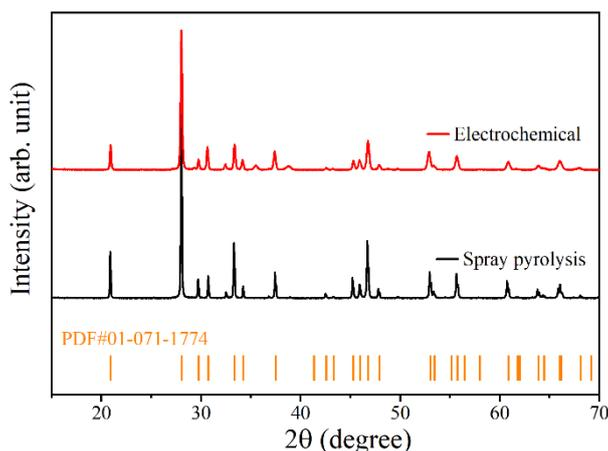
Fig. 1. XRD patterns of  $\text{CuBi}_2\text{O}_4$  fabricated by the electrochemical deposition and spray pyrolysis methods.
