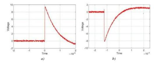
Fig. 4 Lightning impulse - a) Positive polarity; b) Negative polarity.
