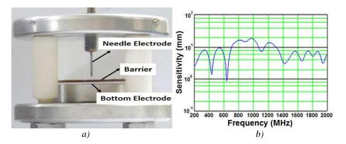
Fig. 5 a) Test cell. b) Frequency response using UHF sensor.
