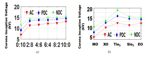
Fig. 6. Corona Inception Voltage under different voltages for different proportions of a) MO and EO; b) MO, XO, XO+Tio<sub>2</sub>, XO+Sio<sub>2</sub>, EO.
