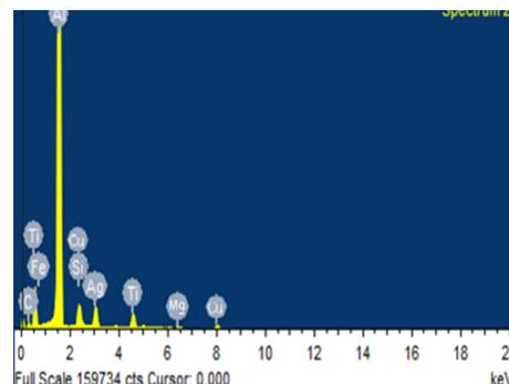
Fig. 2. EDS graph of A356 + SiC + Gr.
