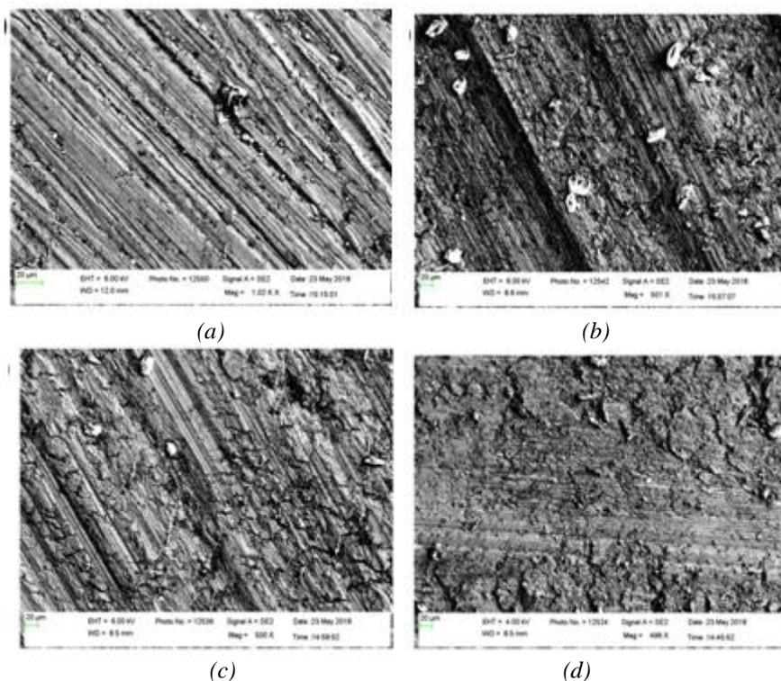
Figs. 6 Worn surface for S4 Test a) at 10 N, b) at 5 N load, c) at 1000 SD d) at 3000m SD.
