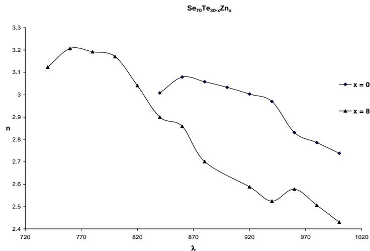
Fig.2 Variation of refractive index ( $n$ ) with wave length ( $\lambda$ ) in  $\text{Se}_{70}\text{Te}_{30}$  and  $\text{Se}_{70}\text{Te}_{22}\text{Zn}_8$  thin films
