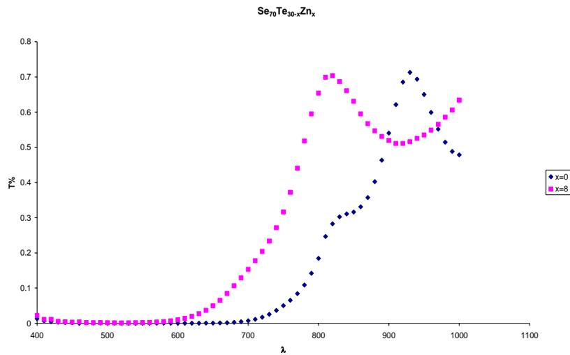
Fig. 1 Variation of transmittance ( $T$ ) with wavelength ( $\lambda$ ) in  $\text{Se}_{70}\text{Te}_{30}$  and  $\text{Se}_{70}\text{Te}_{22}\text{Zn}_8$  thin films
