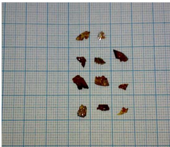
*Fig. 1. As grown crystals of ZnSe.*
