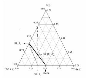
Fig. 3. The ternary phase diagram for Ge-Te-Bi system with the indication of the three pseudo binary composition lines.
