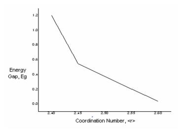
Fig. 2. The plot of the energy gap as a function of the coordination number.
