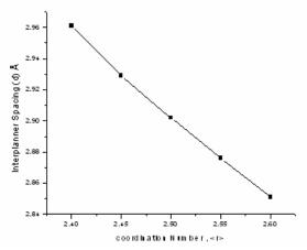
Fig. 1. The plot of the interplanner spacing (d) as a function of the coordination number  $\langle r \rangle$ .
