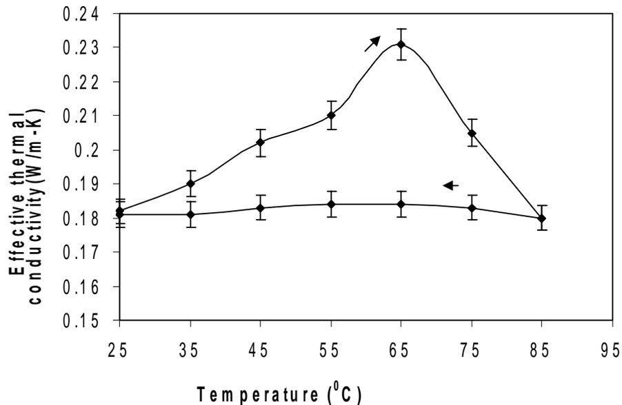
Fig.4 Effective thermal conductivity with different temperature of  $\text{Se}_{81}\text{Te}_{15}\text{Sb}_4$  Chalcogenide glass.
