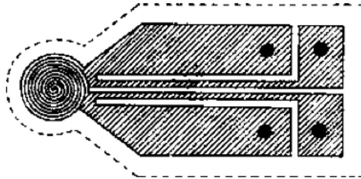
Fig. 1. Schematic diagram of TPS sensor.
