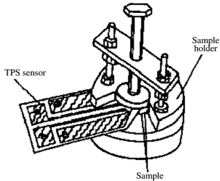
Fig. 2. Sample holder diagram with TPS sensor.
