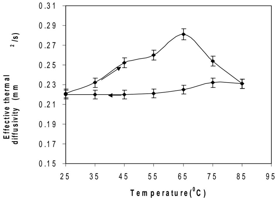
Fig.5 Effective thermal diffusivity with different temperature of  $\text{Se}_{81}\text{Te}_{15}\text{Sb}_4$  chalcogenide glass.
