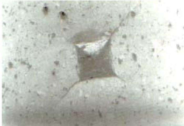
*Fig. 6. Optical Micrographs of typical Indentation Marks on CZR 20 wt% sample sintered at 1400 °C*
