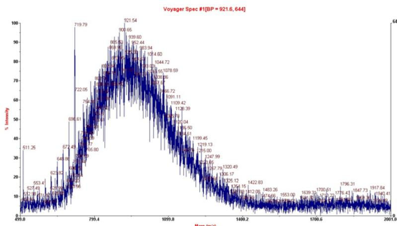
Fig. 1. MALDI TOF mass spectrum of fullereneol  $C_{60}(OH)_{22-24}$ .
