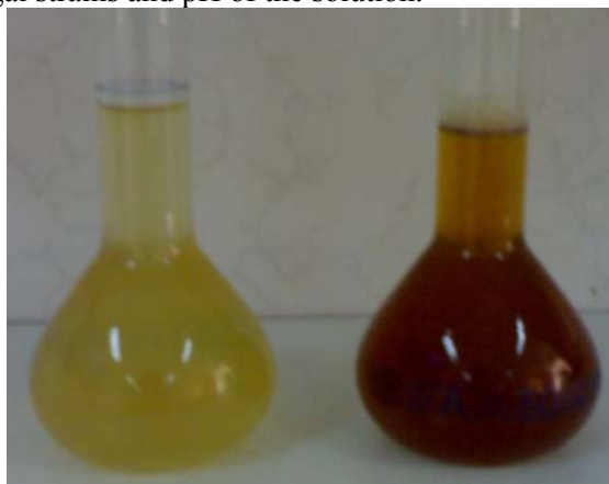
Fig. 1. The color changed from pale yellow to brown arises due to excitation of surface plasmon resonance in the metal nanoparticles indicating the formation of copper NPs.
