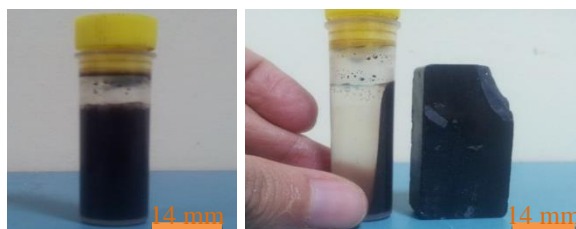
Fig. 2. Observation of the magnetic properties of the nanoparticles before (left) and after (right) placing the magnet
