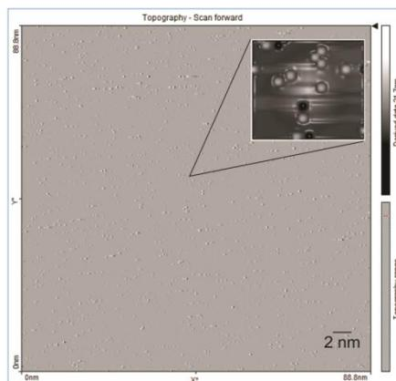
Fig.1. AFM micrographs showing the shape of the  $\text{Ta}_2\text{O}_5$  nanoparticles formed in presence of polysaccharide compound.
