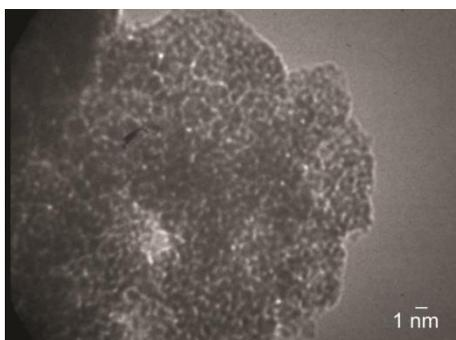
Fig. 4. TEM image of spherical Ta<sub>2</sub>O<sub>5</sub> nanoparticles.
