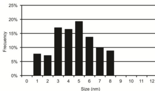
Fig. 2. Particle size distribution of Ta<sub>2</sub>O<sub>5</sub> nanoparticles.
