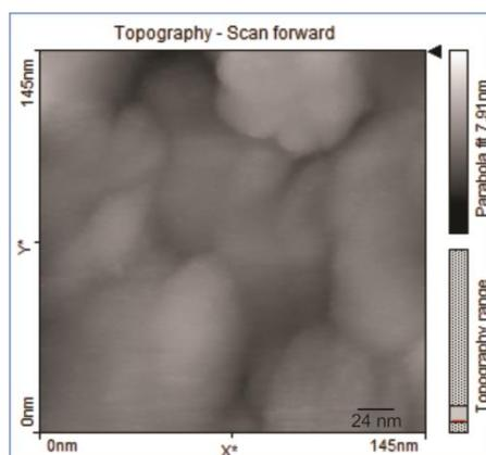
Fig. 3. AFM micrographs showing large Ta<sub>2</sub>O<sub>5</sub> particles of irregular shape formed in absence of polysaccharide compound.
