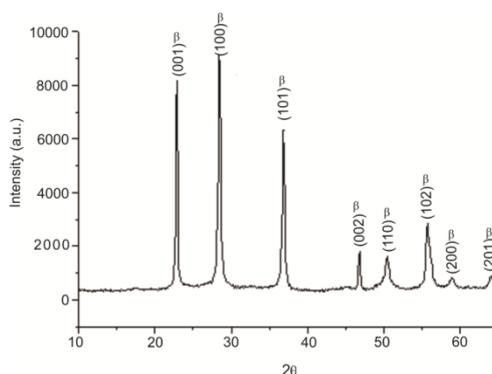
Fig. 6.- X-ray diffraction pattern of sol-gel prepared nanoparticles of  $Ta_2O_5$  calcined at  $800^\circ C$  for 2 h obtained, using a  $CuK(\alpha)$  source at 0.1542 nm.
