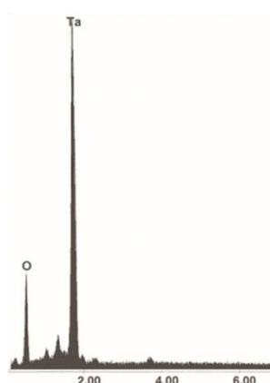
Fig. 5. Typical EDS spectrum of the Ta<sub>2</sub>O<sub>5</sub> nanoparticles obtained.
