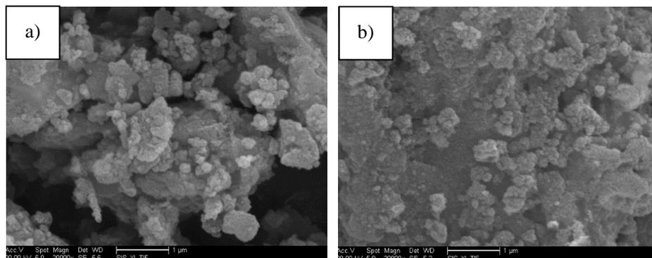
Fig. 5. SEM images of AlN powders with different reaction temperatures: a) 500 °C; b) 550 °C
