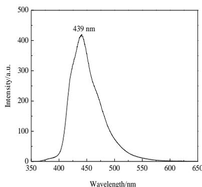
Fig. 3. Photoluminescence spectrum of AlN nanowire
