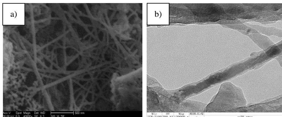
Fig. 2. a). SEM image of AlN nanowire; b) TEM image of local of AlN nanowire
