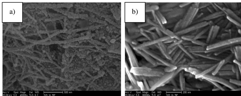
Fig. 7. SEM images of AlN nanowire added different metal ion: a) Mg; b) Zn
