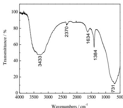
Fig. 4. Infrared spectrum of AlN nanowire
