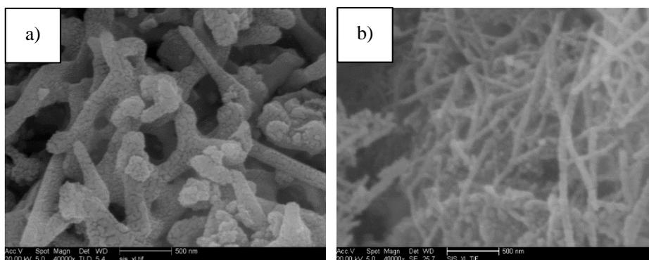
Fig. 8. SEM images of AlN nanowire: a) react without additive; b) additive Mg
