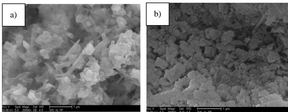
Fig. 6. SEM images of AlN powders with different reaction times: a) 12h; b) 24h
