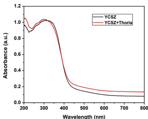
Fig. 5. Typical UV-vis diffuse absorbance spectrum for YCSZ and YCSZ+ThO<sub>2</sub>
