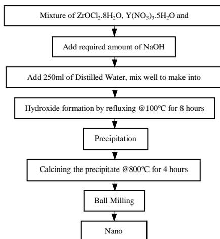
*Scheme 1 Flow chart of the synthesis procedure that was used to prepare stock solutions.*
