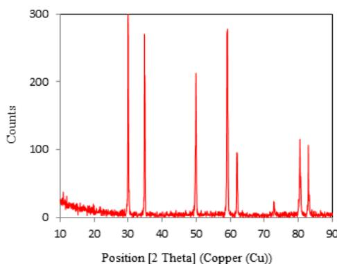
Fig. 4. XRD patterns of as synthesized ceramic
