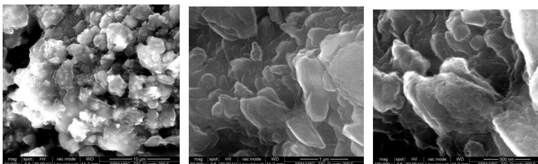
Fig.2 SEM images of synthesized ceramic powder
