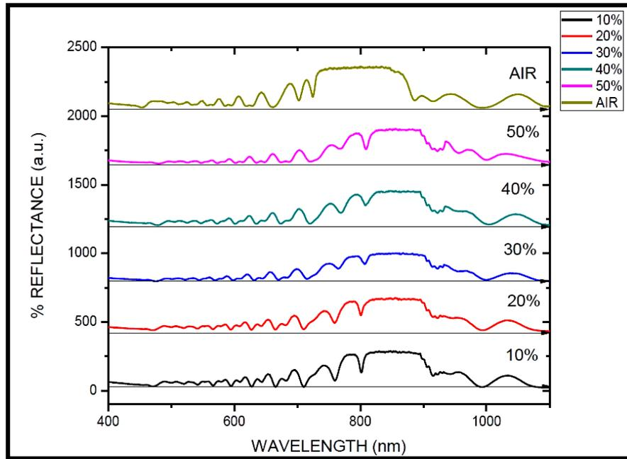
Fig. 5. Reflectance spectra of various concentration of petrol adulterated with kerosene.
