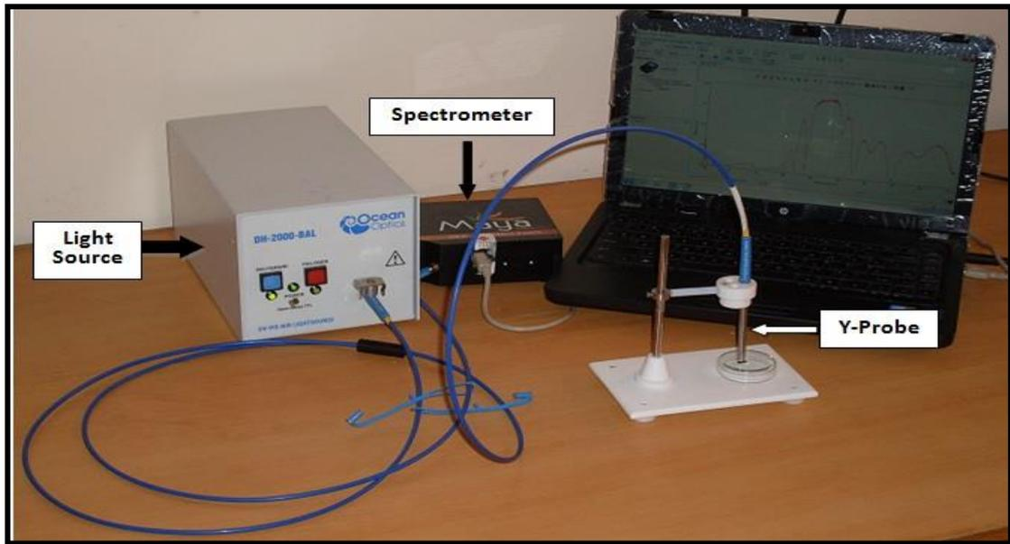
Fig. 2. Optical Spectrometer with Light Source and Accessories
