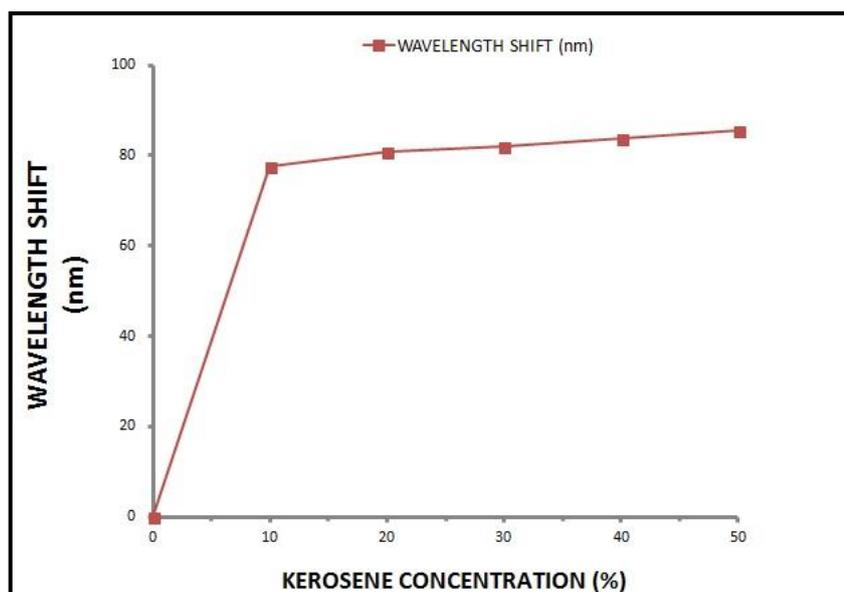
Fig. 6: Wavelength Shift vs Concentration of kerosene.
