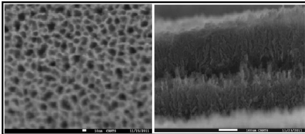
Fig. 3. (a) SEM Plan View of 1D-PSMC Sensor Device (b) SEM Cross-sectional view of Multilayer 1D-PSMC Sensor Device
