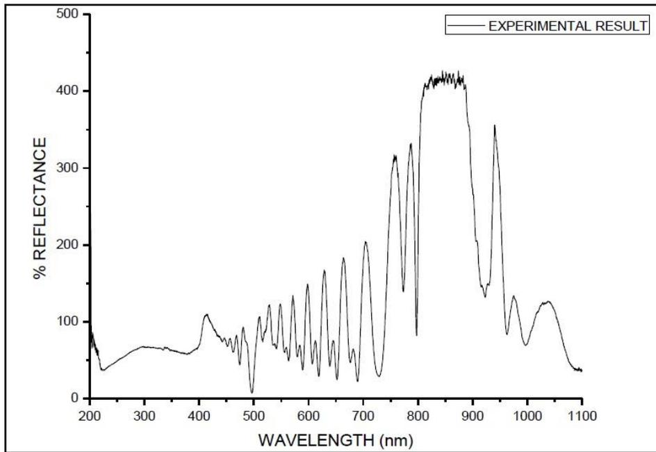
*Fig. 4. Experimental Reflectance Spectra of 1D-PSMC Structure*
