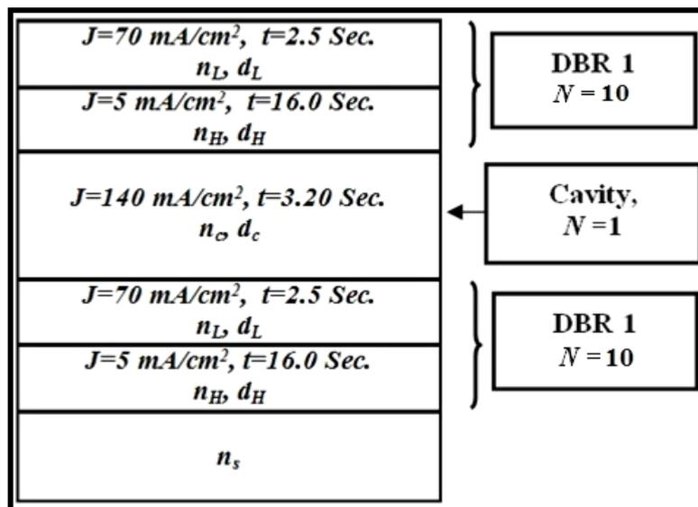
Fig. 1. Fabrication Schematic of 1D-PSMC structures.
