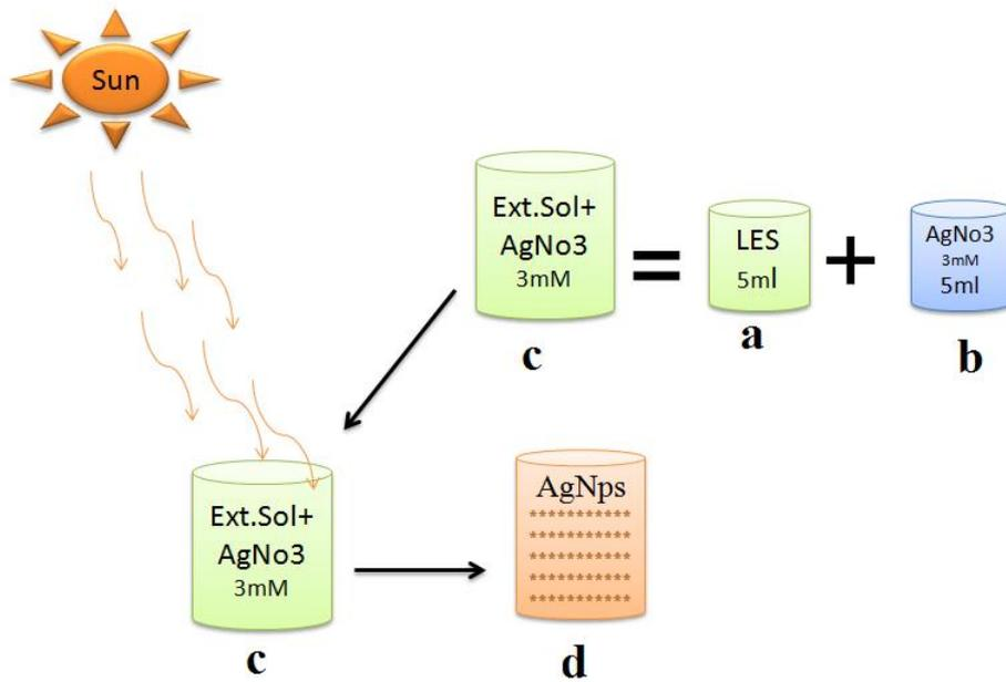
Fig. 8a. Schematic diagram of Photo irradiated-Biosynthesis process of AgNps.
