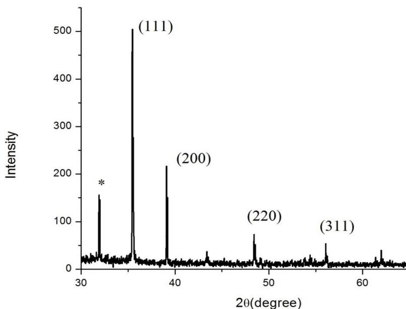
Fig. 6. X-rays diffraction spectrum of the synthesized AgNPs.
