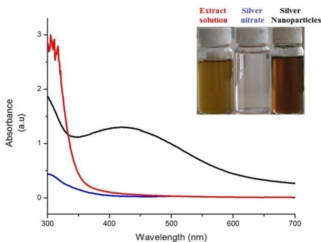
Fig. 2. UV-vis spectra of Photo irradiated-biosynthesized Silver Nanoparticles
