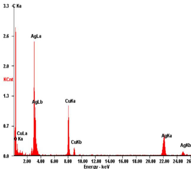
Fig.5. EDAX spectra of photo irradiated-biosynthesized AgNPs
