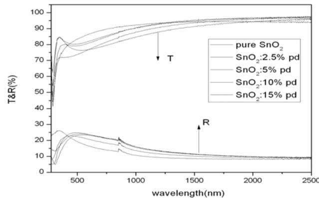
Fig. 3. Optical transmission and reflection for pure  $\text{SnO}_2$  and  $\text{SnO}_2$ :Pd with different concentrations.
