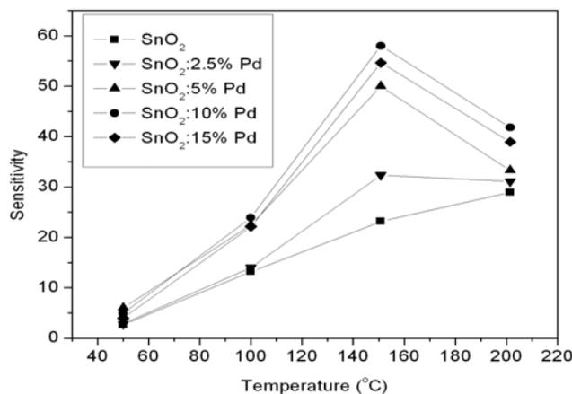
Fig. 5. The CO gas sensitivity of SnO<sub>2</sub> and SnO<sub>2</sub> doped with different Pd concentration versus the operating temperature
