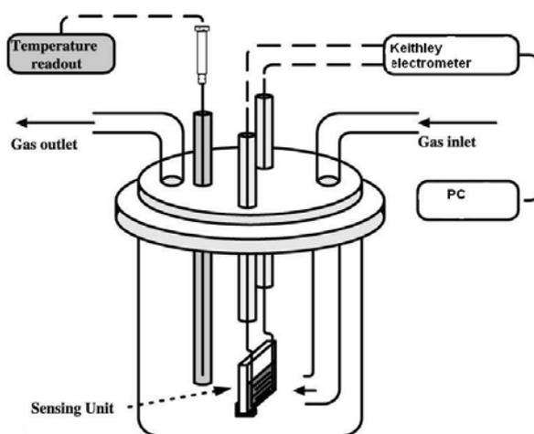
Fig. 1 Gas sensing setup.
