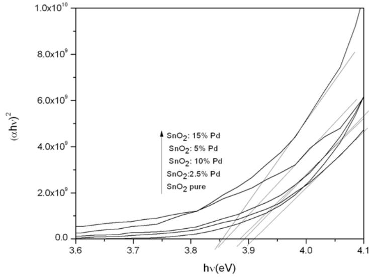
Fig. 4.  $(\alpha hv)^2$  against  $h\nu$  for pure  $\text{SnO}_2$  and  $\text{SnO}_2:\text{Pd}$  with different concentrations.
