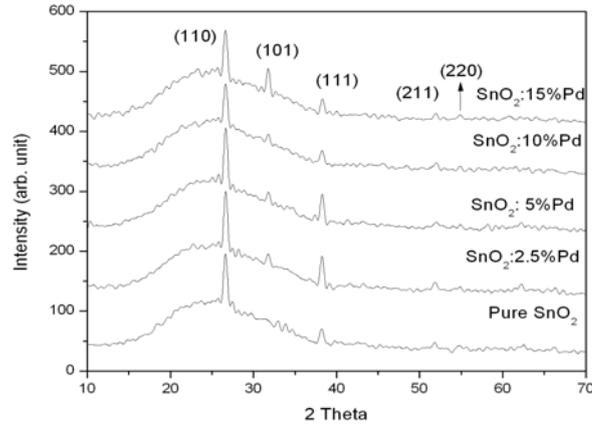
Fig. 2. XRD patterns of pure and  $\text{SnO}_2$  doped with different Pd concentration.
