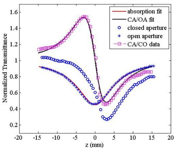
Fig. 7. Normalized Z-scan transmittance curves of the Ag nanoparticle at  $5.889 \times 10^{-3} M$  irradiated with 50 kGy dose. The solid lines are the theoretical fit to the experimental data.
