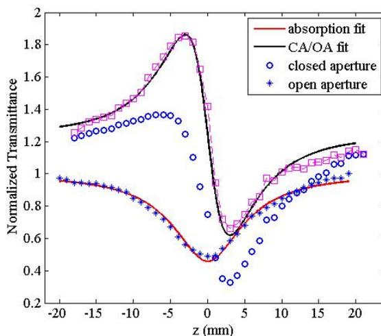
Fig. 6. Normalized Z-scan transmittance curves of the Ag nanoparticle at concentration of  $5.889 \times 10^{-3} M$  irradiated with 40 kGy dose. The solid lines are the theoretical fit to the experimental data.
