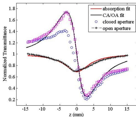
Fig. 5. Normalized Z-scan transmittance curves of the Ag nanoparticle at concentration of  $5.889 \times 10^{-3} M$  irradiated with 30 kGy dose. The solid lines are the theoretical fit to the experimental data.
