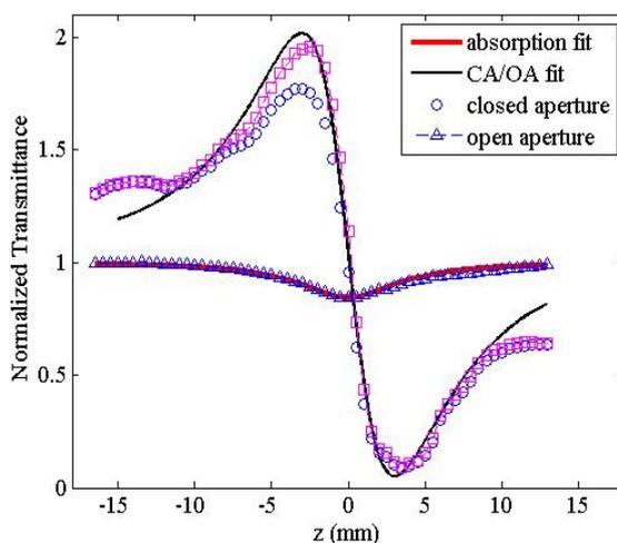
Fig. 3. Normalized Z-scan transmittance curves of the Ag nanoparticle at concentration of  $5.889 \times 10^{-3} M$  irradiated with 10 kGy dose. The solid lines are the theoretical fit to the experimental data.
