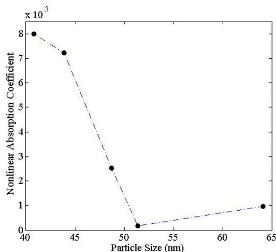
Fig. 9. Nonlinear absorption coefficient plotted as a function of particle size for Ag nanofluid at concentration of  $5.889 \times 10^{-3} M$ .
