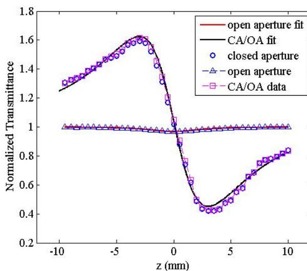
Fig. 4. Normalized Z-scan transmittance curves of the Ag nanoparticle at concentration of  $5.889 \times 10^{-3} M$  irradiated with 20 kGy dose. The solid lines are the theoretical fit to the experimental data.
