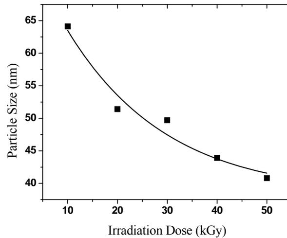
Fig. 1. Variation of particle size of Ag nanofluid ( $5.889 \times 10^{-3} M$ ) at different doses of radiation
