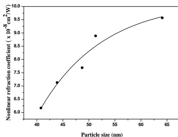
Fig. 8. Nonlinear refraction coefficient plotted as a function of particle size for Ag nanofluid at concentration of  $5.889 \times 10^{-3} M$ .
