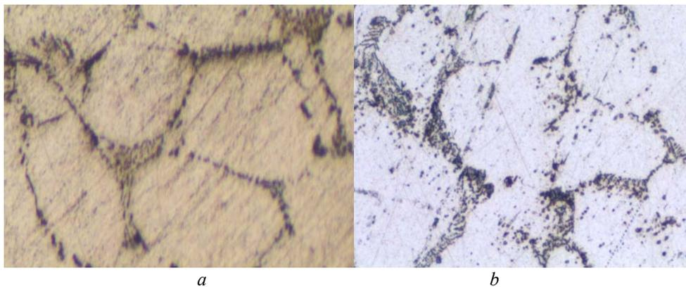
Plate 4- Optical micrograph a) F-Temper b) SHT at 540°C for 1hr 20μm (x200)
