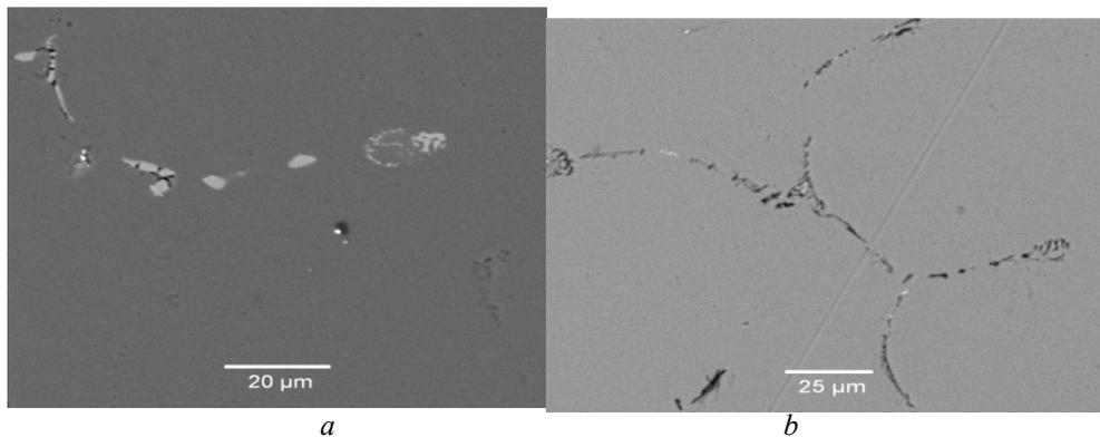
Plate 3- SEM BSE image a) SQA T7 220/20sec, 180/2hr indicating  $Al_8Mg_3FeSi_6$  intermetallic compound b) SEM BSE image IQA<sub>4</sub> with  $Al_3Cr$  dispersoid
