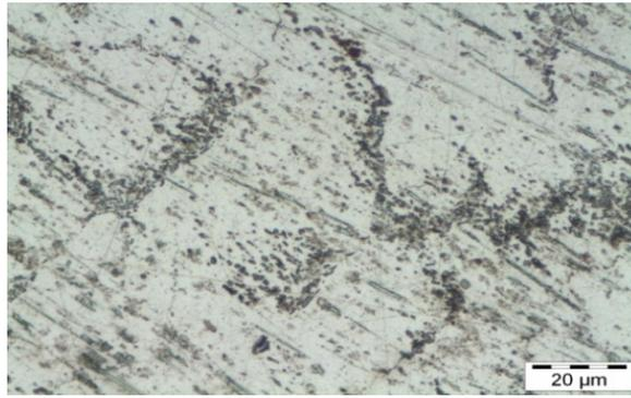
Plate 2- Optical micrograph for STAT peak aged at 180°C/2hr
