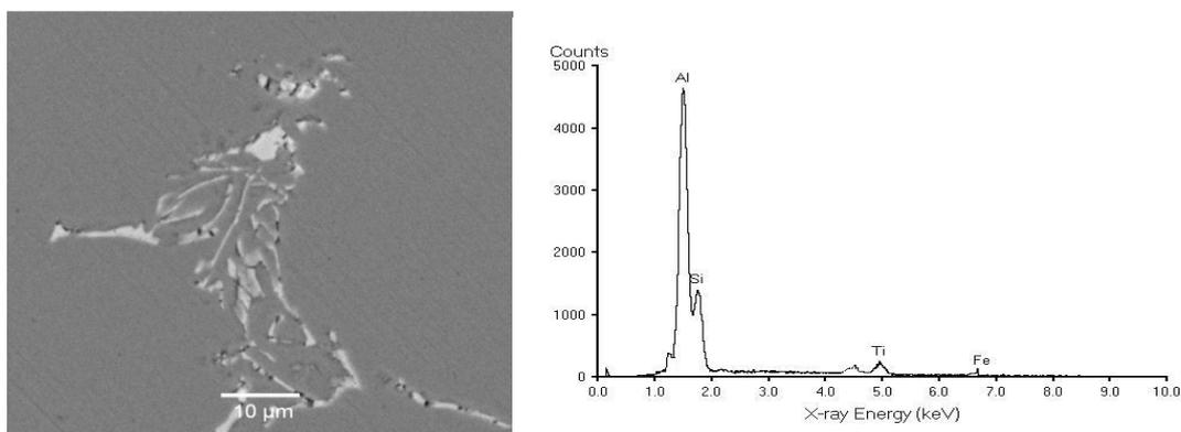
Plate 1- SEM micrograph of T7 180°C/20hr with the EDS spectrum showing  $\beta''Mg_2Si$  and  $Al_{12}Mg_{17}$ .
