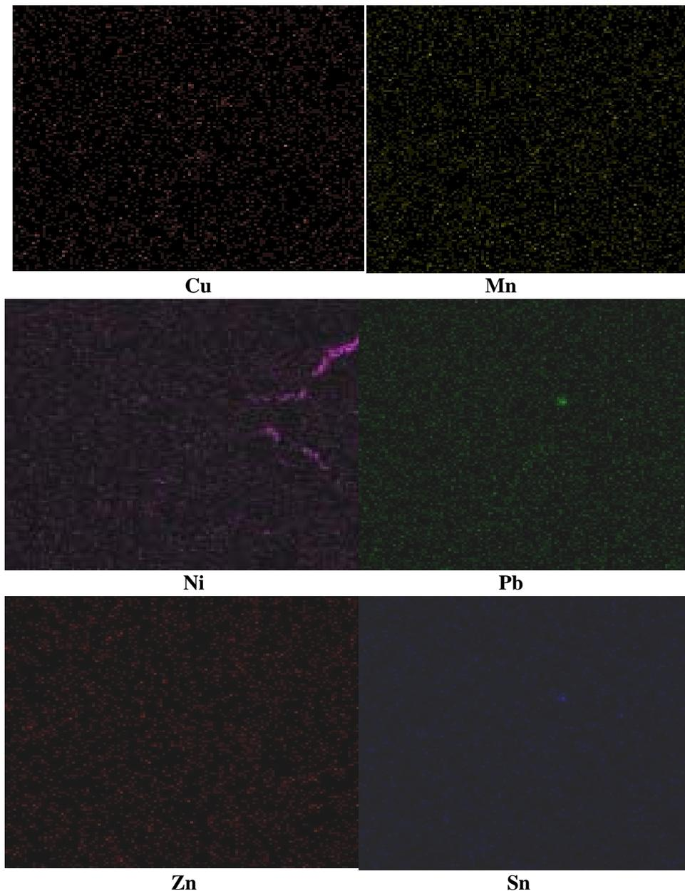
*Plate 5- SEM-EDS mapping for peak-aged DTAT A356.0-type Al-Si-Mg sample at 180/20hr with Fe, Ti, Cr, Cu, Mn, Ni, Pb, Zn and Sn element.*
