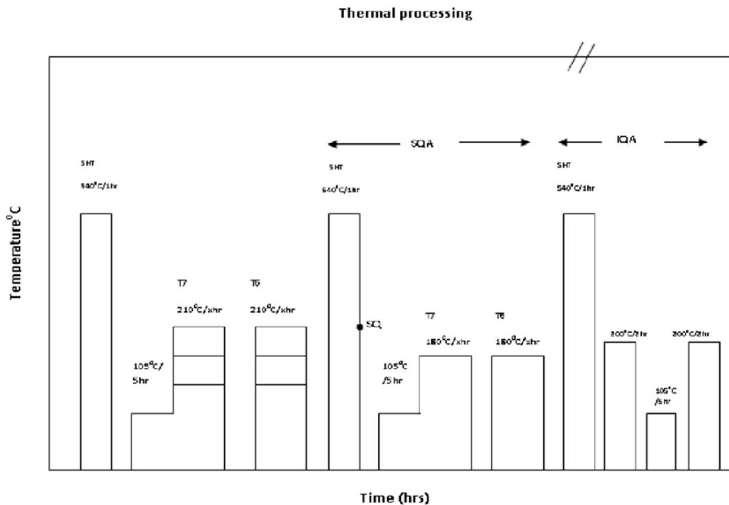
Fig. 1- Schematic diagram of the isothermal treatments used for Al-Si-Mg alloy
