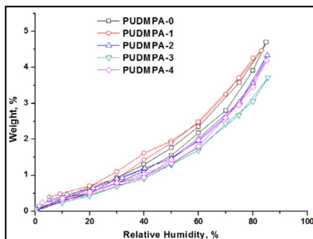
Fig. 2. Sorption/desorption isotherms of polyurethane membranes modified by nano-ZnO
