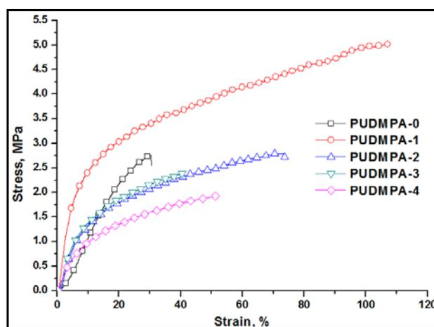
Fig. 4. Stress-strain measurements of polyurethane membranes modified by nano-ZnO
