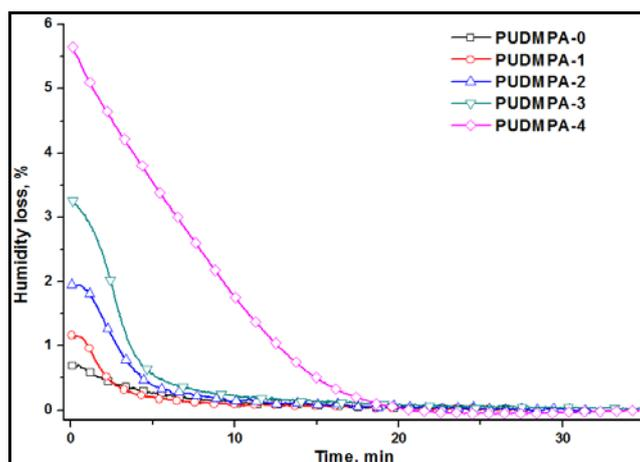
Fig. 3. Drying kinetic curves of polyurethane membranes modified by nano-ZnO
