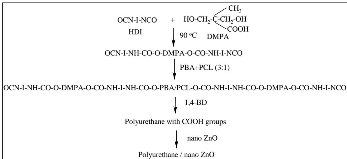
*Scheme 1. Synthetic route for obtaining of polyurethane membranes modified by nano-ZnO*
