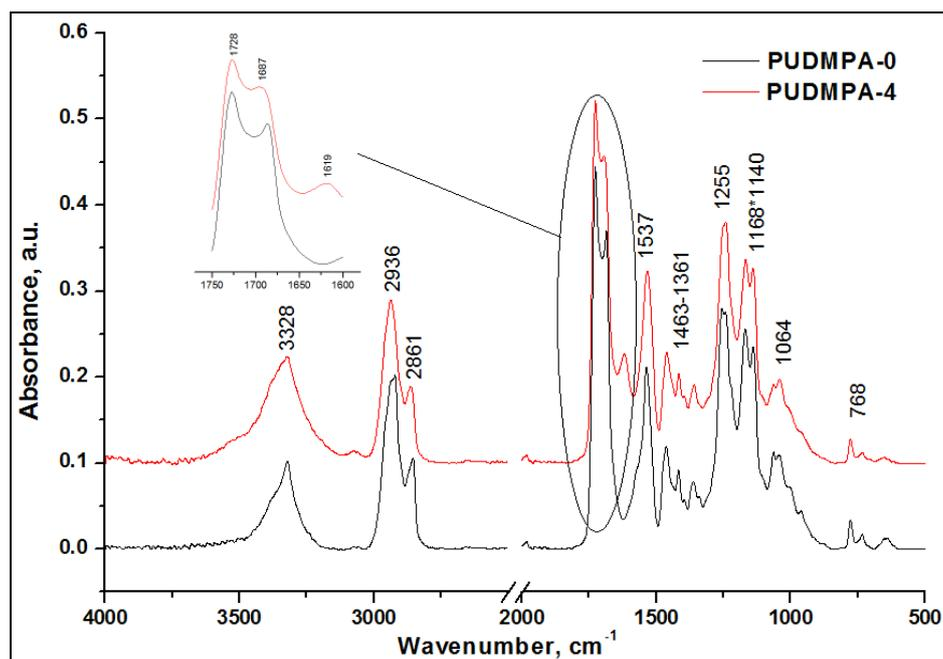
*Fig.1. Representative ATR-FTIR spectra of the blank polyurethane sample and respectively polyurethane membrane modified by nano-ZnO*
