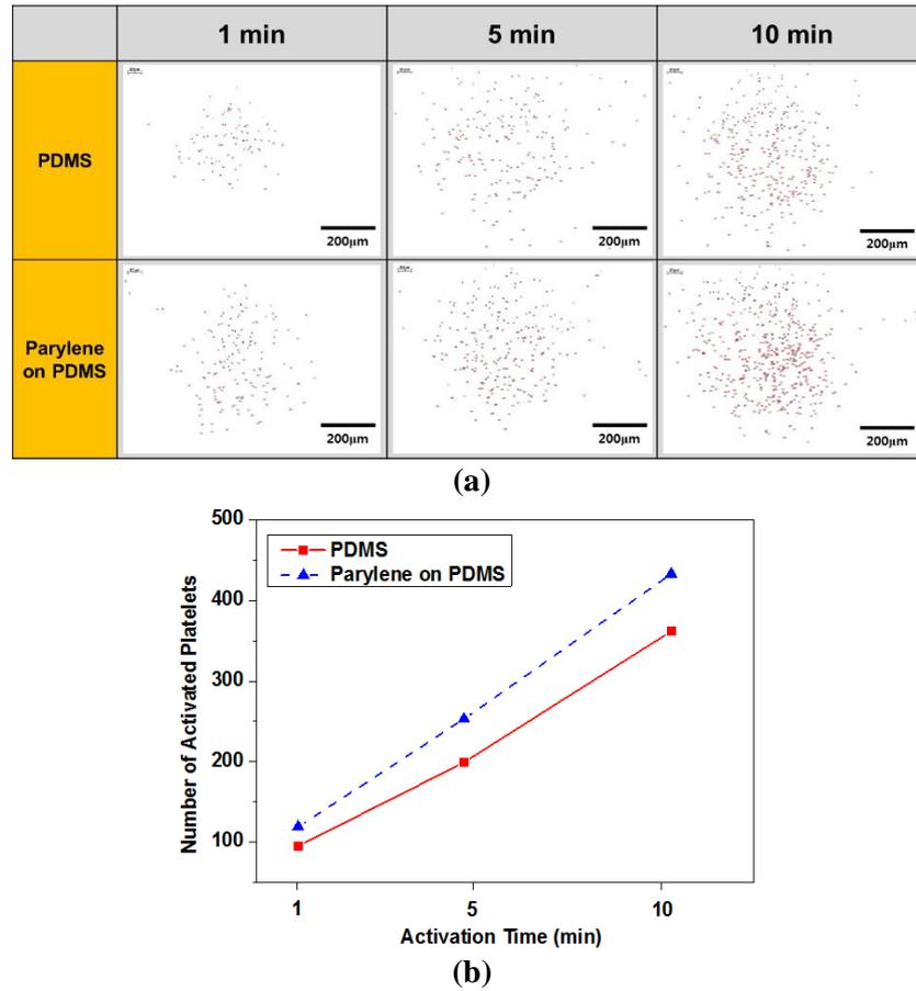
Fig. 3. (a) Fluorescent images of the activated platelets stained with P-selectin and (b) the graph showing the number of activated platelets on the PDMS and parylene-on-PDMS substrates with time (1, 5, and 10 minutes), respectively.
