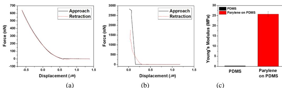
Fig. 2. Force-displacement curves of (a) PDMS, (b) parylene on PDMS recorded from approach to retraction of a cantilever, and (c) Young's moduli obtained at retraction from force-displacement curves.
