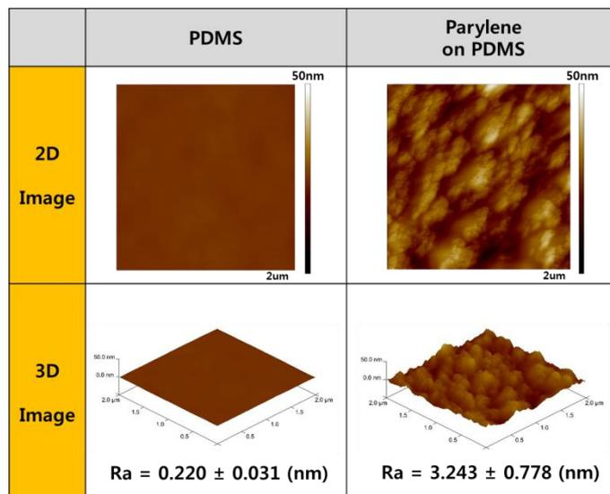
Fig. 4. Roughness of the PDMS and parylene-on-PDMS substrates measured with an atomic force microscope (AFM).
