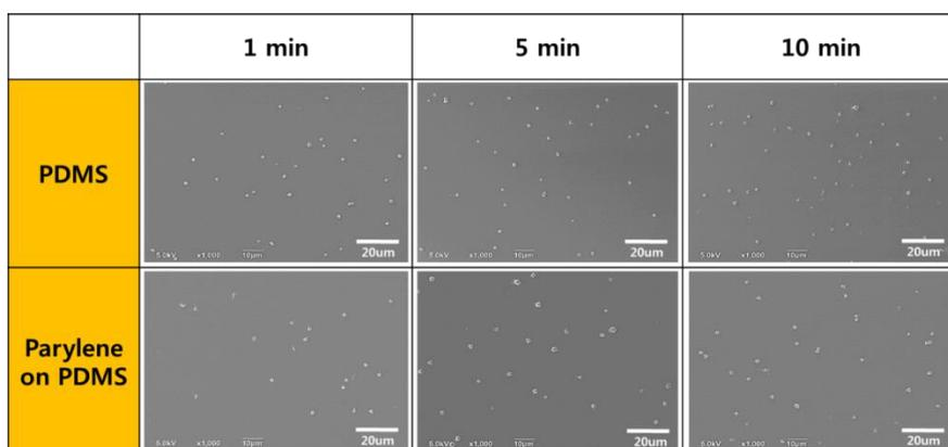
Fig. 1. High-resolution scanning electron microscopic images of platelet attachments according to the PDMS and parylene-on-PDMS substrates with time (1, 5, and 10 minutes).
