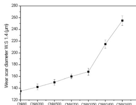
Fig. 3. Wear scar diameters for tribological investigation of CNWs coated steel disks in the presence of SAE 20 base oil as lubrication medium.
