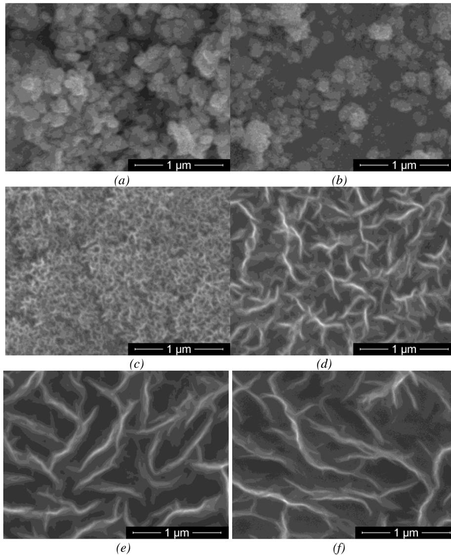
*Fig. 1. Morphology of (a) CNW200, (b) CNW500 and (c) CNW700 (d) CNW1050 and (e) CNW1400 and (f) CNW1600 coated disk samples.*
