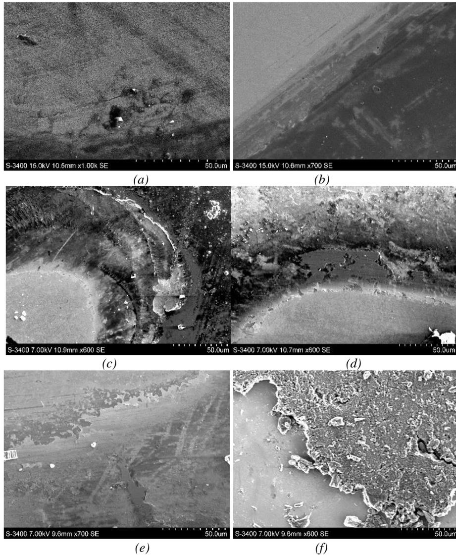
Fig.4. Morphology of (a) CNW200, (b) CNW500 and (c) CNW700 (d) CNW1050 and (e) CNW1400 and (f) CNW1600 coated disk samples after tribological investigations.
