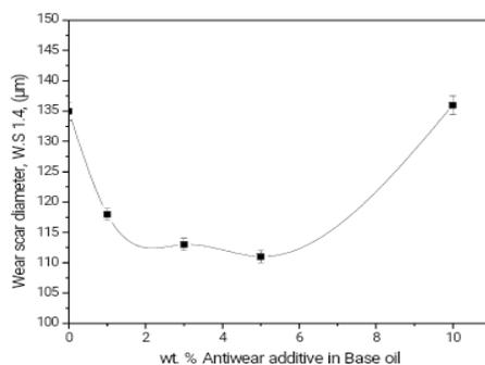
Fig. 6. Wear scar diameters for tribological investigation of uncoated steel disks in the presence of SAE 20 base oil additivated with AW additive, as lubrication medium.
