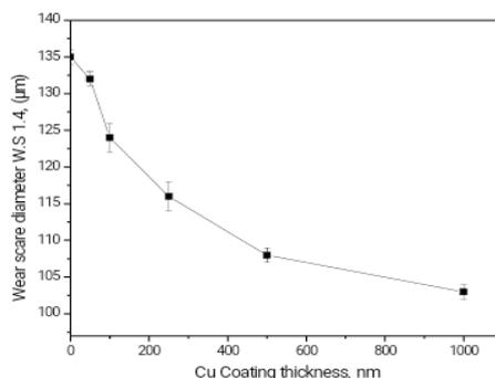
Fig. 5. Wear scar diameters for tribological investigation of Cu coated steel disks in the presence of SAE 20 base oil as lubrication medium.
