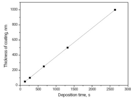
Fig. 2. Influences of the deposition time on thickness of the copper coating.
