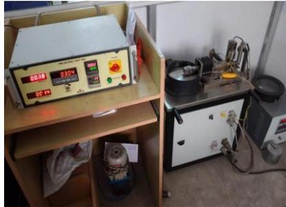
Fig. 5. Wear Testing Machine.
