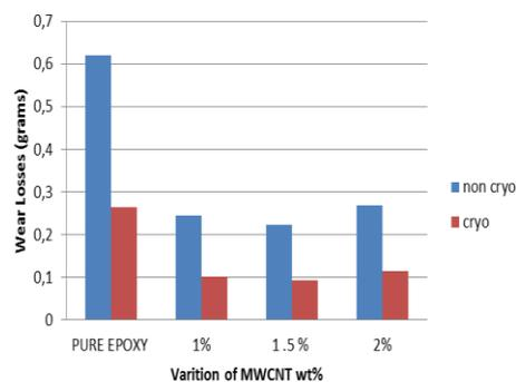
Fig.6.Losses of cryogenic and non cryogenic treated samples at 10N.
