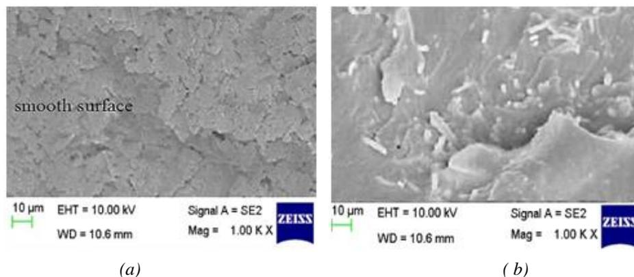
Fig. 4. a) Untreated 1.5 weight % MWCNT and  $\text{Al}_2\text{O}_3$ , b) Cryogenic treated 1.5 Weight % MWCNT and  $\text{Al}_2\text{O}_3$ .
