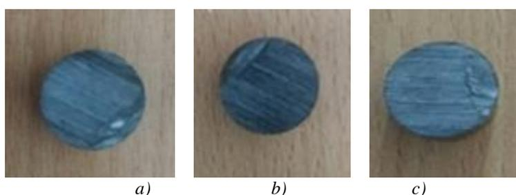
Fig. 1. Wear Tested Samples of (a) 1 % weight ratio of MWCNT and Al<sub>2</sub>O<sub>3</sub>, (b) 1.5 % weight ratio of MWCNT and Al<sub>2</sub>O<sub>3</sub> (c) 2 % weight ratio of MWCNT and Al<sub>2</sub>O<sub>3</sub>.
