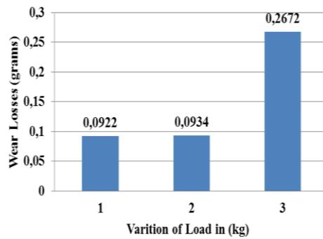
Fig. 9. Wear losses of cryogenically treated 1.5wt% sample at various loads.
