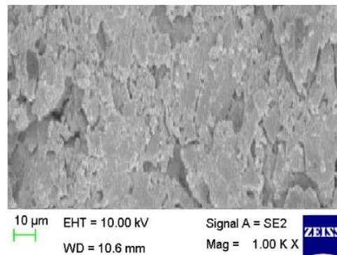
Fig. 3. SEM image of cryogenically treated pure epoxy.
