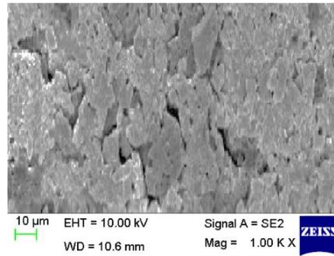
Fig.2. SEM Image of untreated pure epoxy.
