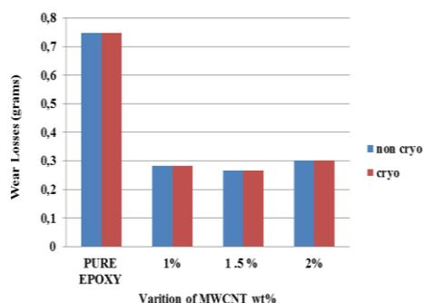
Fig. 8. Losses of cryogenic and non cryogenic treated samples at 30N.
