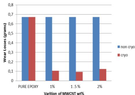
Fig. 7. Wear losses of cryogenic and non cryogenic treated samples at 20N.
