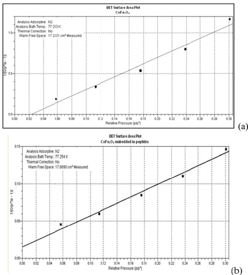
Fig. 5. BET plot using points collected at the pressure range 0.05 to 0.3 by the BET equation used to determine the surface area for  $\text{CoFe}_2\text{O}_4$  (a) and  $\text{CoFe}_2\text{O}_4$ /dipeptide (b)
