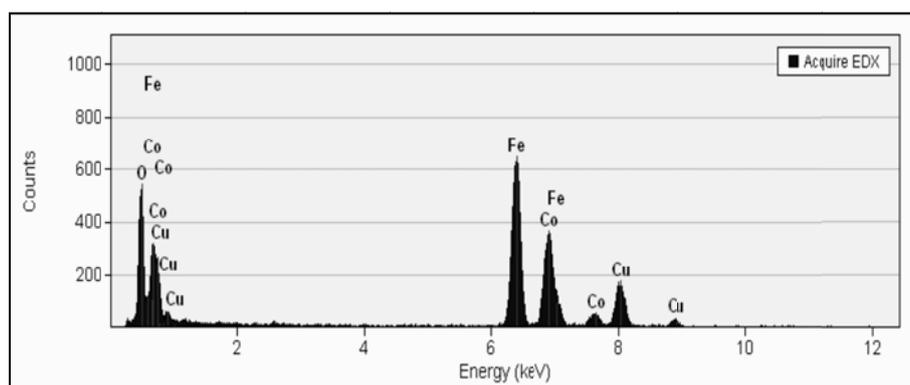
Fig. 3. EDX spectrum for  $\text{CoFe}_2\text{O}_4$
