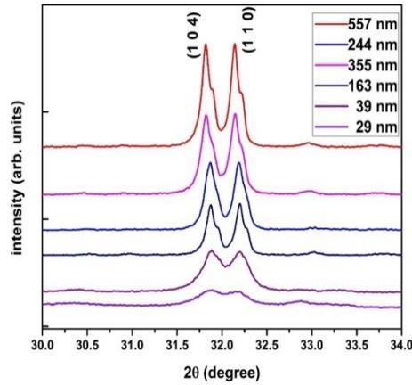
Fig.2. Peak broadening of Bragg peaks with respect to crystallite size
