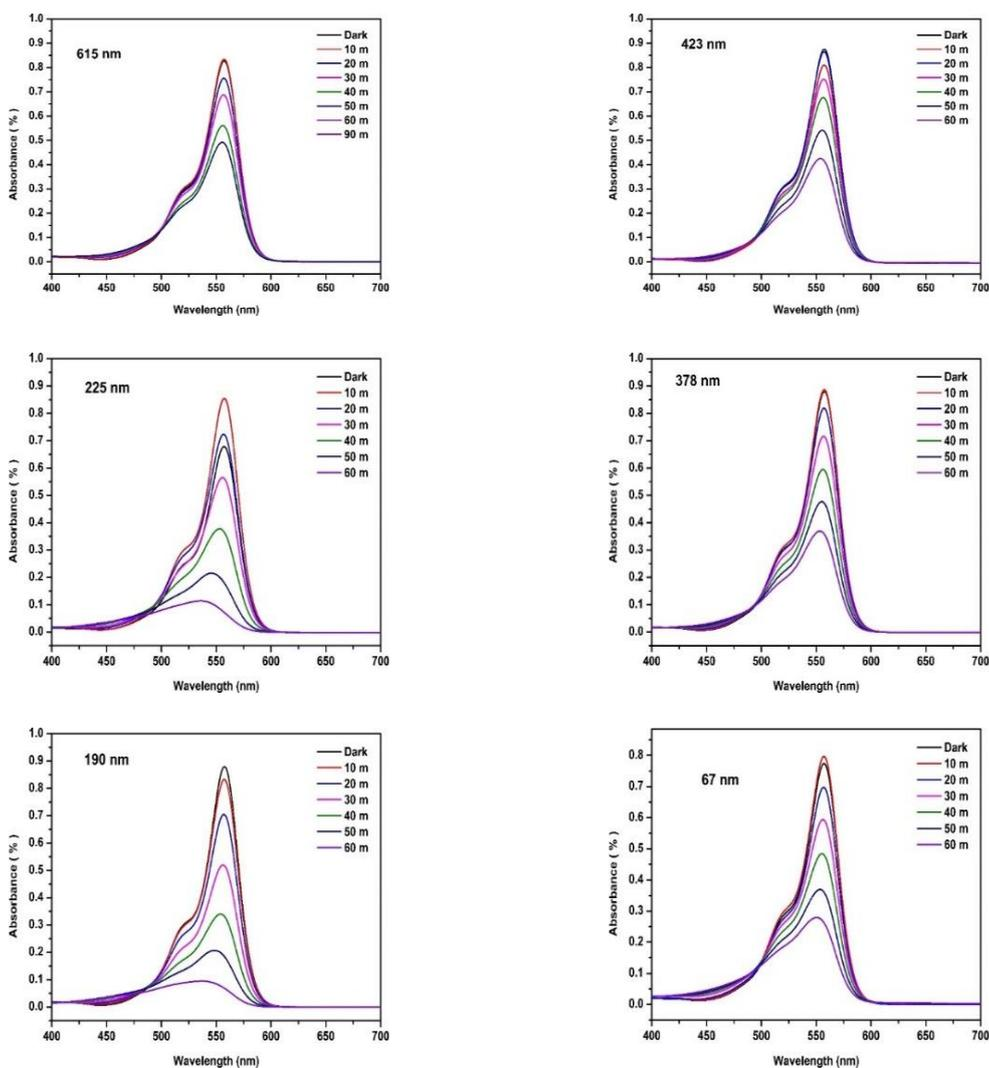
Fig.6. Absorption spectra of RhB with respect to time in presence of BFO photocatalyst of different grain sizes under visible light irradiation
