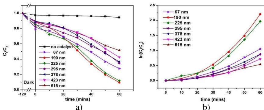
Fig.7. (a) Photo degradation and (b) Photo degradation kinetics of RhB in presence of BFO photocatalyst
