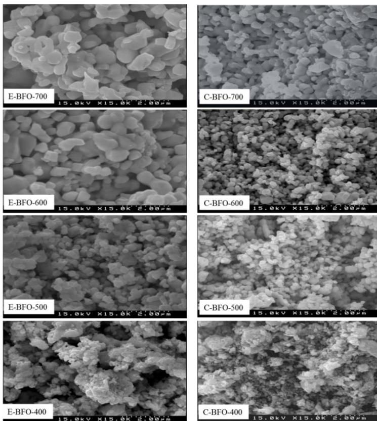
Fig.3. SEM profiles of prepared BFO particles
