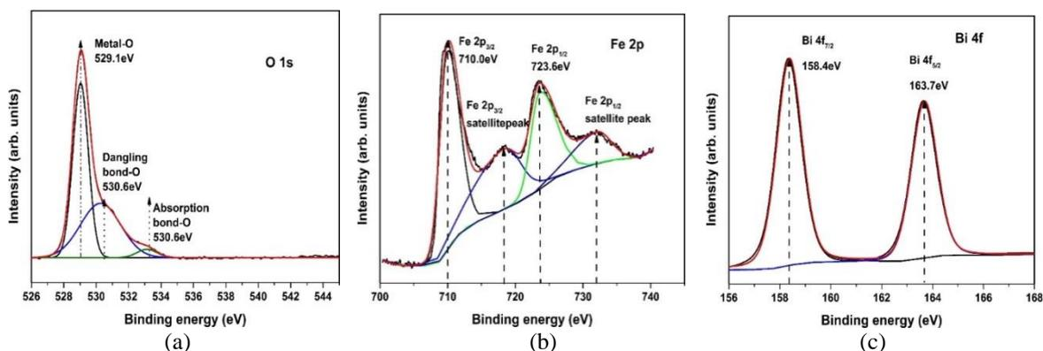
Fig.4. XPS narrow scan spectra of (a) Fe 2p (b) O 1s (c) Bi 4f states of BFO particles with grain size 190 nm.
