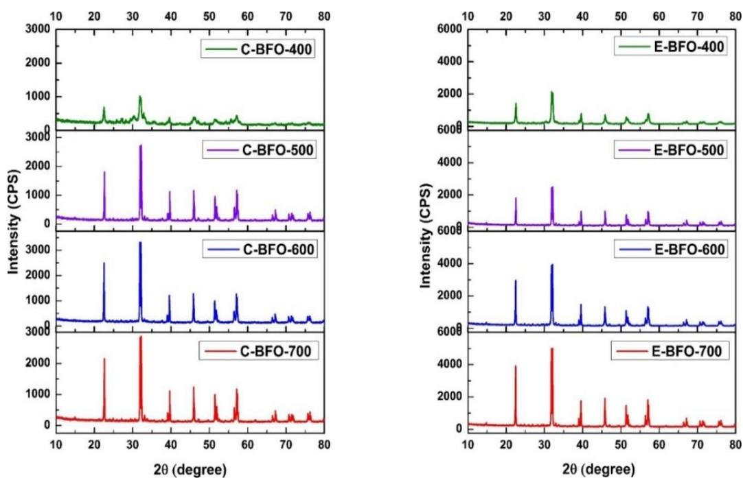
Fig.1. XRD profiles of prepared BFO particles
