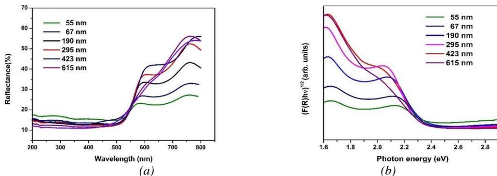
Fig.5. (a) Dependence of reflectance with grain size of BFO particles and (b) corresponding plots of  $(F(R)h\nu)^{1/2}$  Vs  $h\nu$
