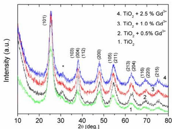
Fig. 1. XRD patterns of pure and  $Gd^{3+}$  doped  $TiO_2$  nanoparticles.
