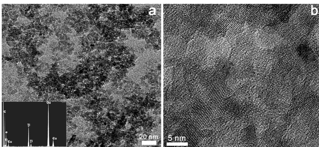
Fig. 2. Typical TEM images, low (a) and high (b) magnification, of  $TiO_2$  nanoparticles doped with 2.5at%  $Gd^{3+}$  ions. Inset: EDS data.
