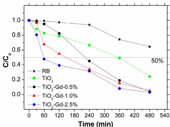
Fig. 4. Effect of different photocatalysts on the degradation of RB. Initial concentration of RB was  $10^{-5}$  M; concentration of catalyst was 1 mg/ml. For comparison photolysis of RB is also presented.
