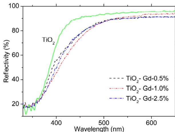
Fig. 3. UV/vis reflectance spectra of pure  $\text{TiO}_2$  and  $\text{TiO}_2$  doped with different at.% of  $\text{Gd}^{3+}$  ions.
