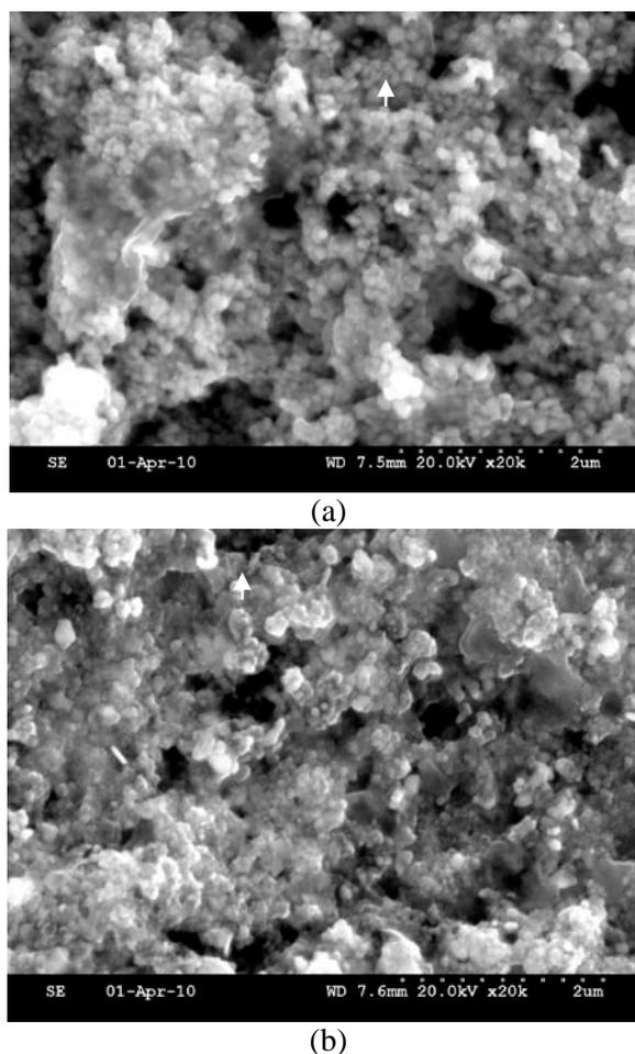
Fig. 3. SEM micrograph of silver nanoparticles synthesized by plant extracts (particles shown by arrow of 30 nm)- a) *E.hirta* b) *N.indicum*
