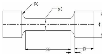
Fig.2 Tensile specimen size
