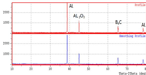
Fig 4. XRD Analysis of the hybrid composites
