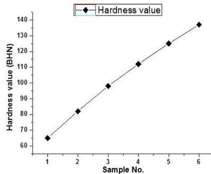
Fig. 6 Brinell values of hybrid composites
