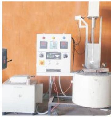
*Fig.1 Stir Casting Setup*
