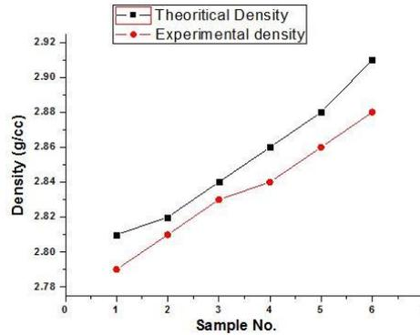
Fig. 5 Theoretical and Experimental density values of composites
