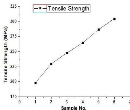
Fig. 6 Tensile strength values of hybrid composites
