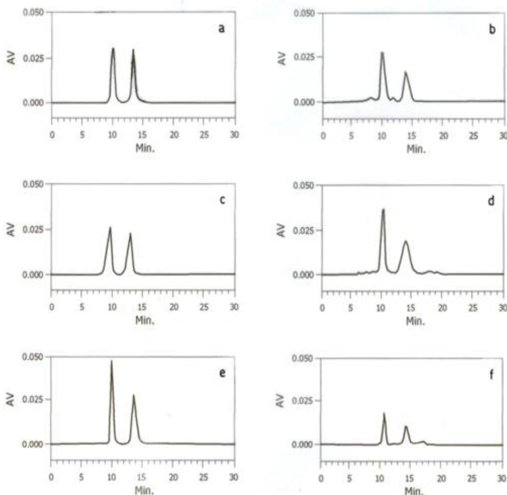
Fig. 3. Typical HPLC chromatograms of DP enantiomers, (a) pure bulk sample, (b) in 0.1 N HCl after 48 h, (c) in 0.1 N NaOH after 48 h, (d) in 3% H<sub>2</sub>O<sub>2</sub> after 48 h. (e) under UV light after 10 d, (f) at 60°C after 10 d.
