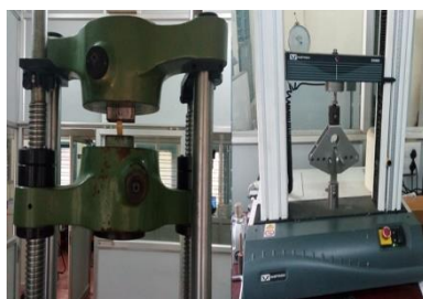
Fig. 2. Photographic image of tensile and flexural testing machine.
