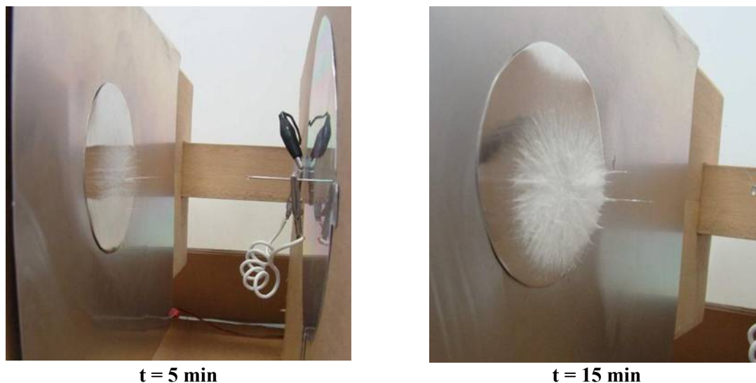
t = 5 min t = 15 min Fig. 5. Photographs of spontaneous formation of yarns from fibers prepared by electrospinning of solutions from \text{PCA}_5\text{D}_1/\text{P}(\text{AMPS-co-TBA}) containing 0.40 mol/L NaCl, electrospinning time: 5 or 15 min; total polymer concentration: 25 wt.%.
