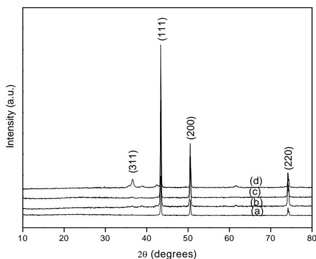
Fig. 2. X-ray diffraction pattern of Copper dendrite like structure (a) as prepared, (b) 200°C, (c) 400°C and (d) 600°C annealed samples.
