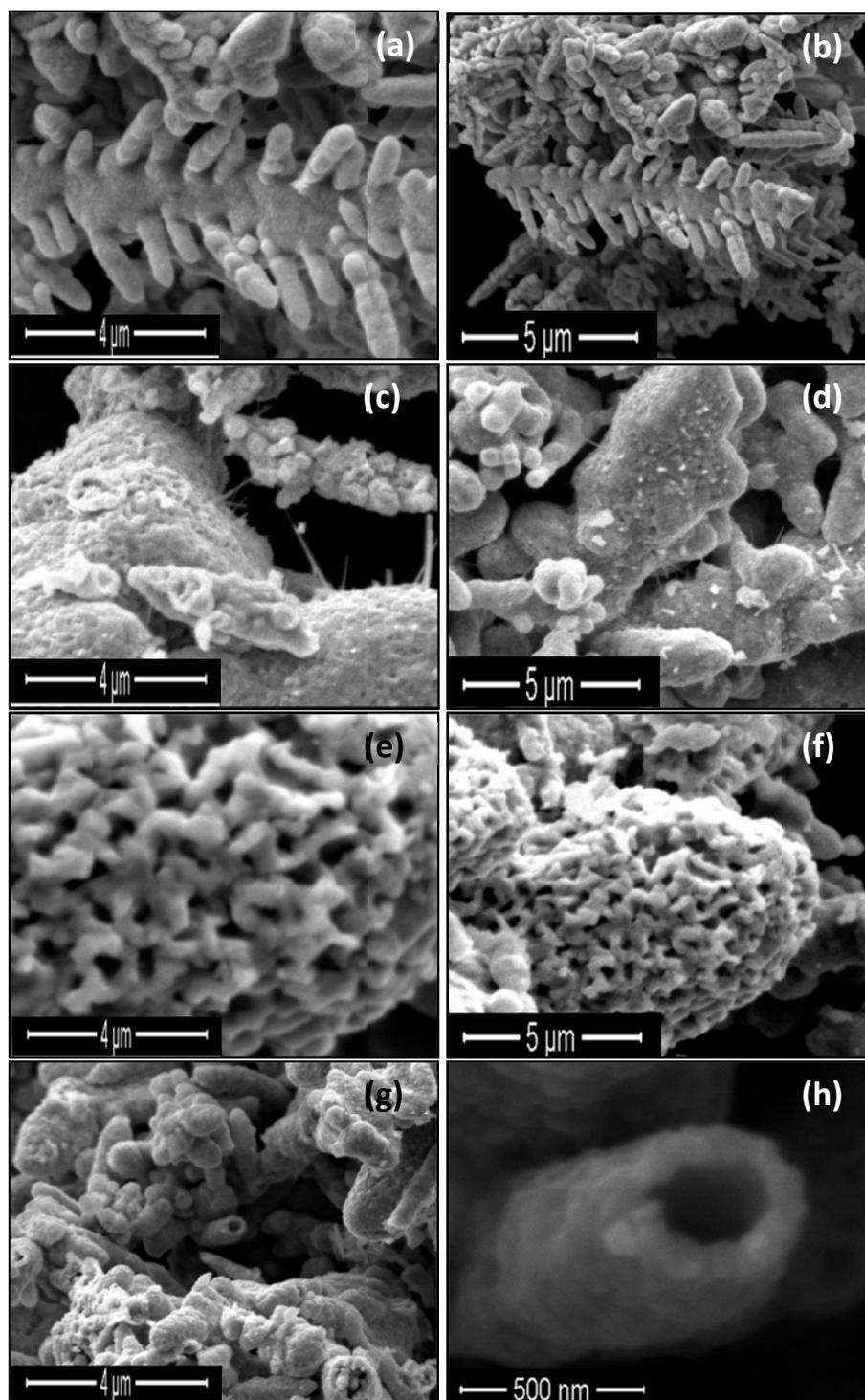
Fig. 2. SEM images of copper (a, b) as prepared and annealed at (c, d) 200°C, (e, f) 400°C, (g, h) 600°C
