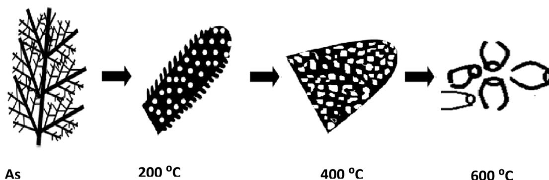
Fig. 4. Schematic description of the growth process of hierarchical copper structures.
