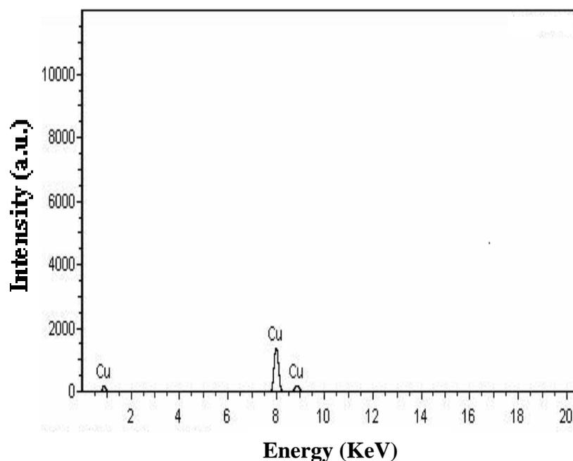
*Fig. 3. EDX spectra of copper.*
