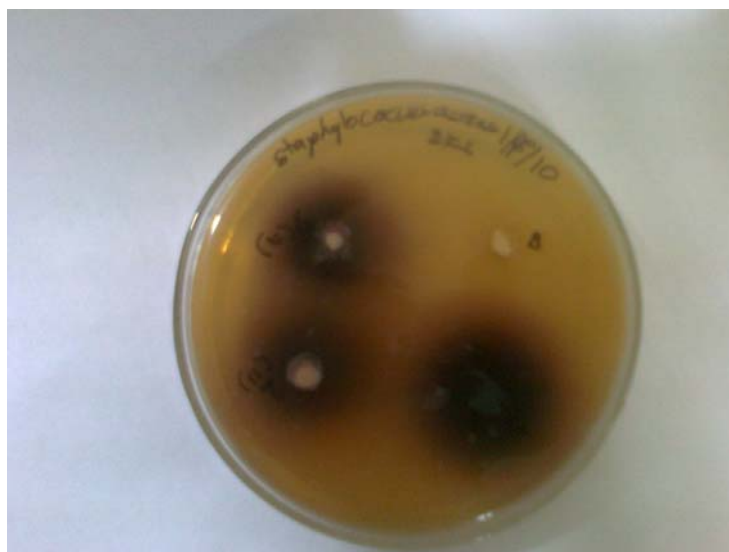
Fig. 12. Zone of inhibition of particles synthesized by wet chemical method. Index: Top left - iron oxide nanoparticles, Bottom left Iron-Cobalt nanoparticles and bottom right – Zero valent nanoparticles
