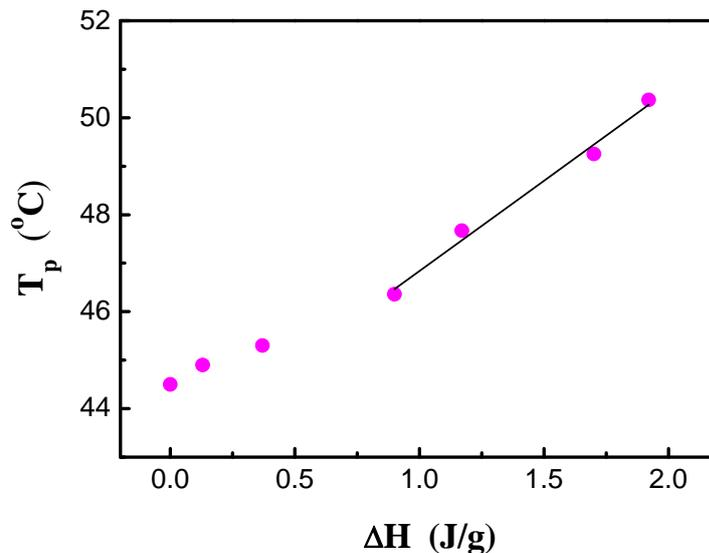
Fig. 6 Variation of the endothermic peak temperature  $T_p$  with the enthalpic loss  $\Delta H$ . The full line represents a least-squares fitting to data points corresponding to higher aging times.
