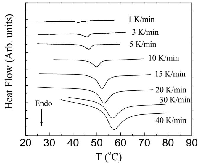
Fig. 1 DSC curves obtained for  $Bi_5Se_{95}$  chalcogenide glass at heating rates varying between 1 and 40 K/min. Only endothermic outputs are shown.
