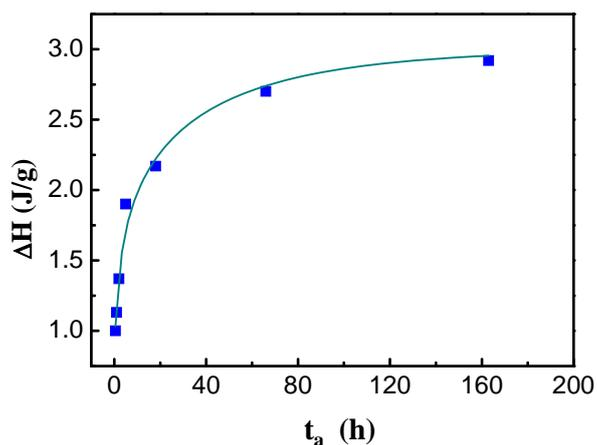
Fig. 5  $\Delta H$  versus  $t_a$  for glassy  $\text{Bi}_5\text{Se}_{95}$ . The annealing temperature is 300 K. The solid line is the theoretical fit to the Cowie-Ferguson equation.
