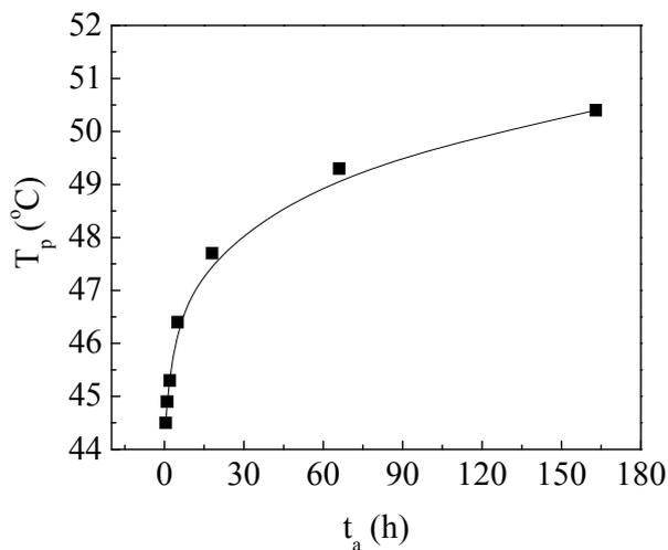
Fig. 4 The variation of peak temperature  $T_p$  with  $t_a$  for glassy  $\text{Bi}_5\text{Se}_{95}$ . The annealing temperature is 300 K. The solid line is a guide to the eye.
