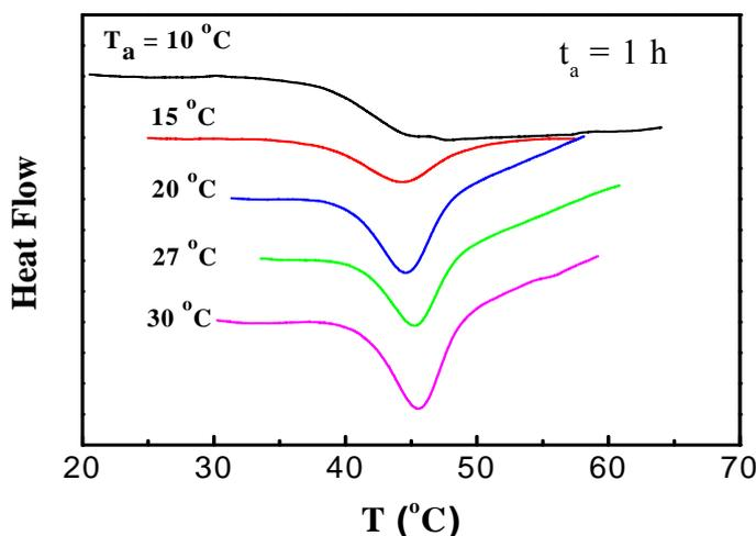
Fig. 7 DSC curves obtained for glassy  $\text{Bi}_5\text{Se}_{95}$  at aging time  $t_a = 1$  h for various aging temperatures and for heating rate of 10 K/min.
