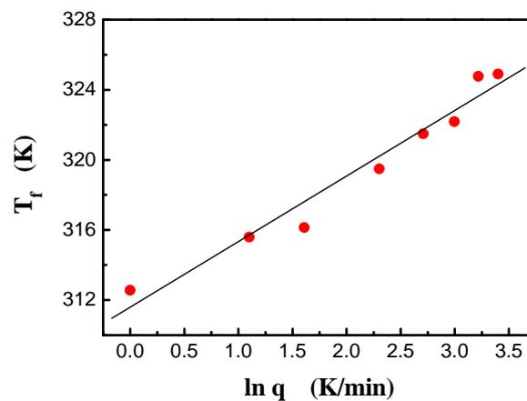
Fig. 2 Lasocka plot of the dependence of the limiting fictive temperature  $T_f$  on  $\ln q$ . The solid line represents fit to Eq.3.
